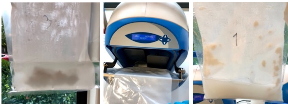
Figure 3.15. Left: Blender bag containing sample and 0,85 % peptone salt diluent, ready to be homogenized. Middle: Open blender SMASHER® (AES blueline, bioMérieux, France). The picture shows how the blender bag is placed inside the blender, and the plates used to beat the bag homogenizing the content. Right: Blender bag with sample already homogenized.
