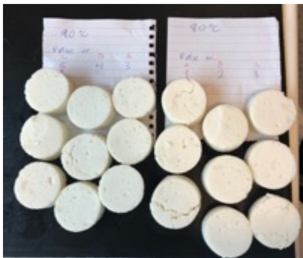
Figure 4.1.6 Fish mince samples from the potato starch variants heat-treated using the two different time and temperature combinations in the preliminary production after TPA was performed. Samples to the left was from the variant heat-treated at 90 °C for 10 min, samples to the right were from the variant heat-treated at 80 °C for 30 min.
