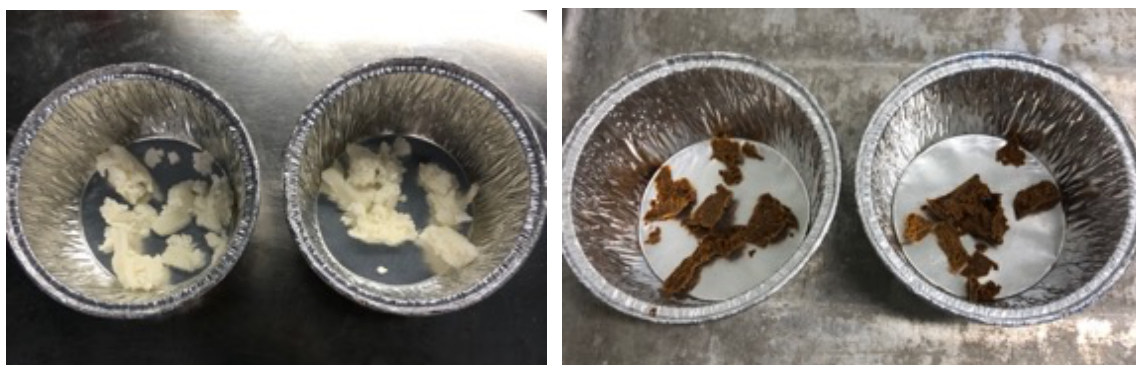
Figure 3.10. Aluminium containers with fish mince samples before (left) and after (right) drying for 18-22 h at 105\text{ }^{\circ}\text{C} .
