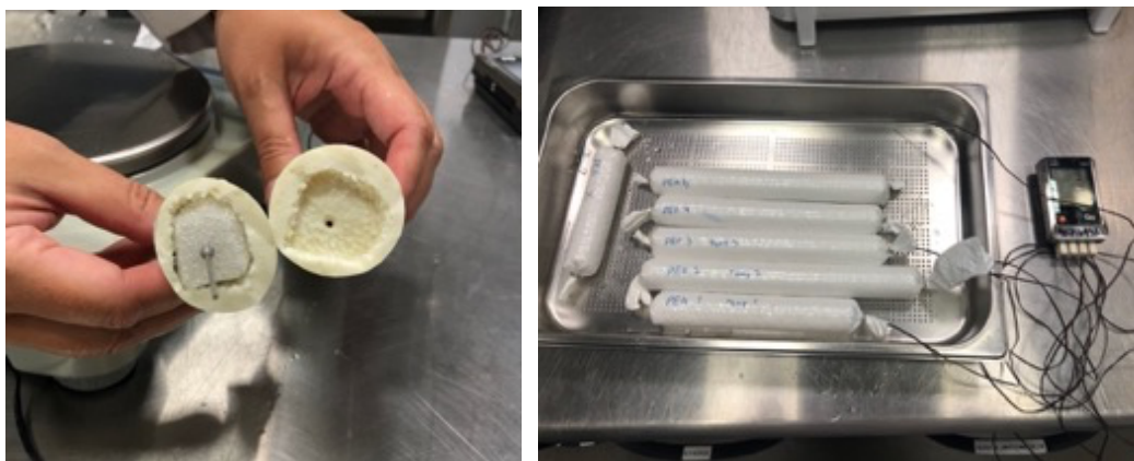
Figure 3.5. Left: A temperature probe cut out from a heat-treated sample. The hole in the sample shows where the probe was positioned during heat treatment. Right: Temperature probes inside three different samples with cords attached to the data storage device (Testo 176T4, Testo SE & Co, KGaA, Germany).
