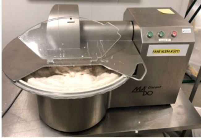
Figure 3.12. Mixed fish mince inside the industrial cutter (MTK 662, MADO GmbH, Germany) used in the production for the shelf-life study.
