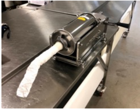
Figure 3.4. The manual sausage stuffer (Model 5 Litre De Luxe, Tre Spade, Italy) used to stuff the fish mince into casings.
