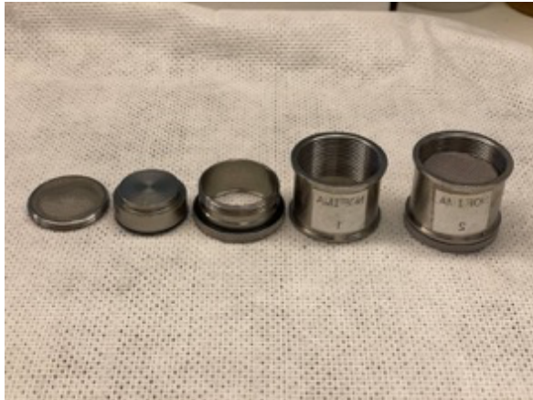
Figure 3.8. Sample cups used to measure the water holding capacity of the fish mince. From left: filter, two bottom pieces, the cup itself, already assembled sample cup.
