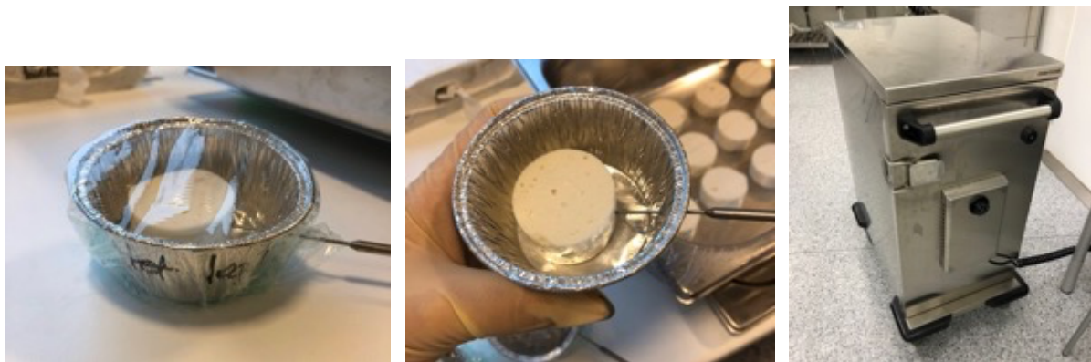
Figure 3.14. Left: Temperature probe inside a sample in an aluminium container wrapped in plastic wrap. Middle: A temperature probe penetrated through an aluminium container into a sample. Right: The food warming trolley used to keep the samples warm until analysis (Termia 950 H, Metos, Finland).
