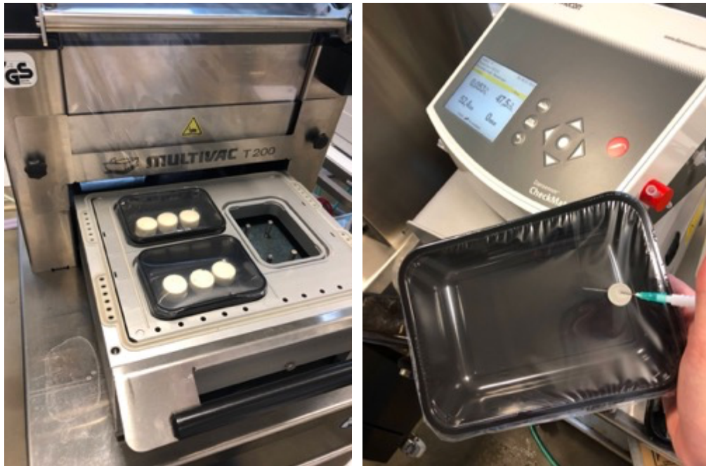
Figure 3.13. Left: Modified atmosphere packing machine with finished sealed packages containing three sample pieces each. Right: A random sample check of the atmosphere inside the packages.
