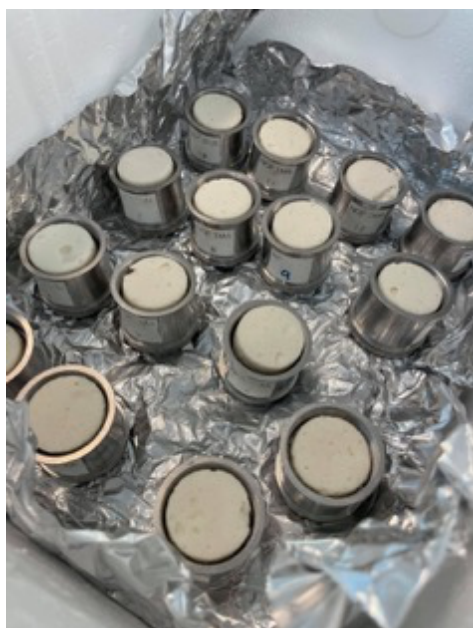
Figure 3.9. Samples of fish mince in the sample cups prepared for WHC analysis.
