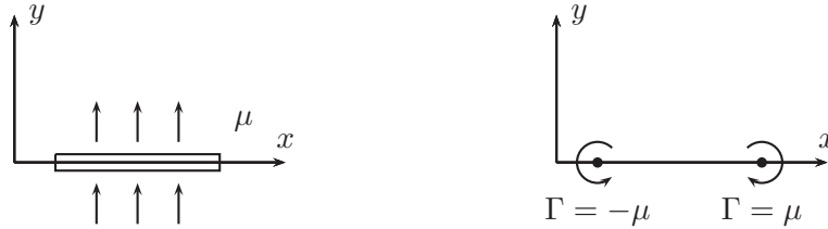
Figure 5.3: The constant doublet element is similar to two point vortices, and will give the same velocities in the far-field.
