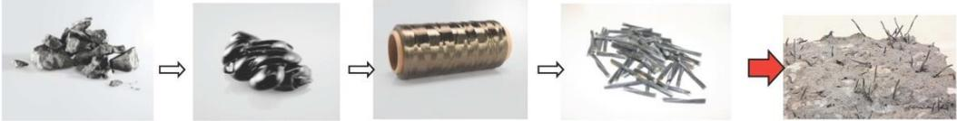
Basalt stone      Melted Basalt      Fiber      MiniBars™      Pre-Reinforced Concrete
