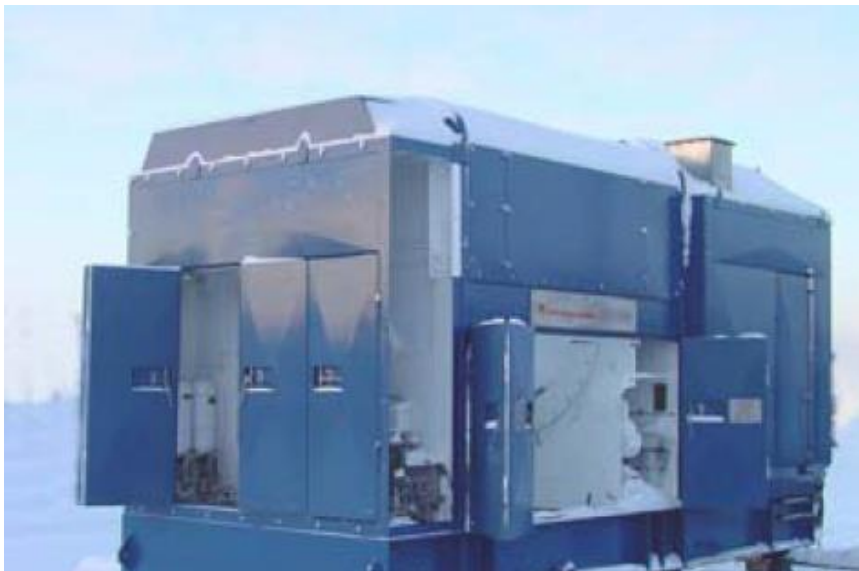
Figure 48 AHD mainframe and enclosure of main parts (National Oilwell Varco, 2006)
