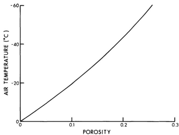
Figure 6.5: Air temperature at which it would be possible for rubble of porosity \gamma to completely consolidate. Note that the initial temperature distribution in the ice sheet is assumed as linear and equal to the air temperature on the top surface (Kry, 1977).
