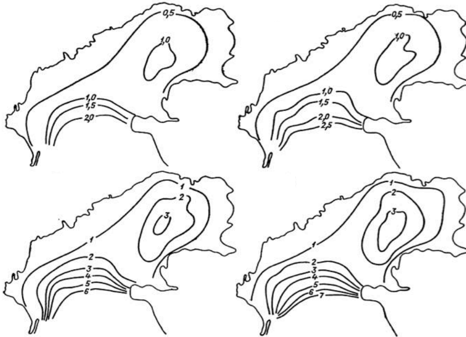
Figure 3.9: Significant and maximal wave heights for different return periods (Terziev et al., 1992):
