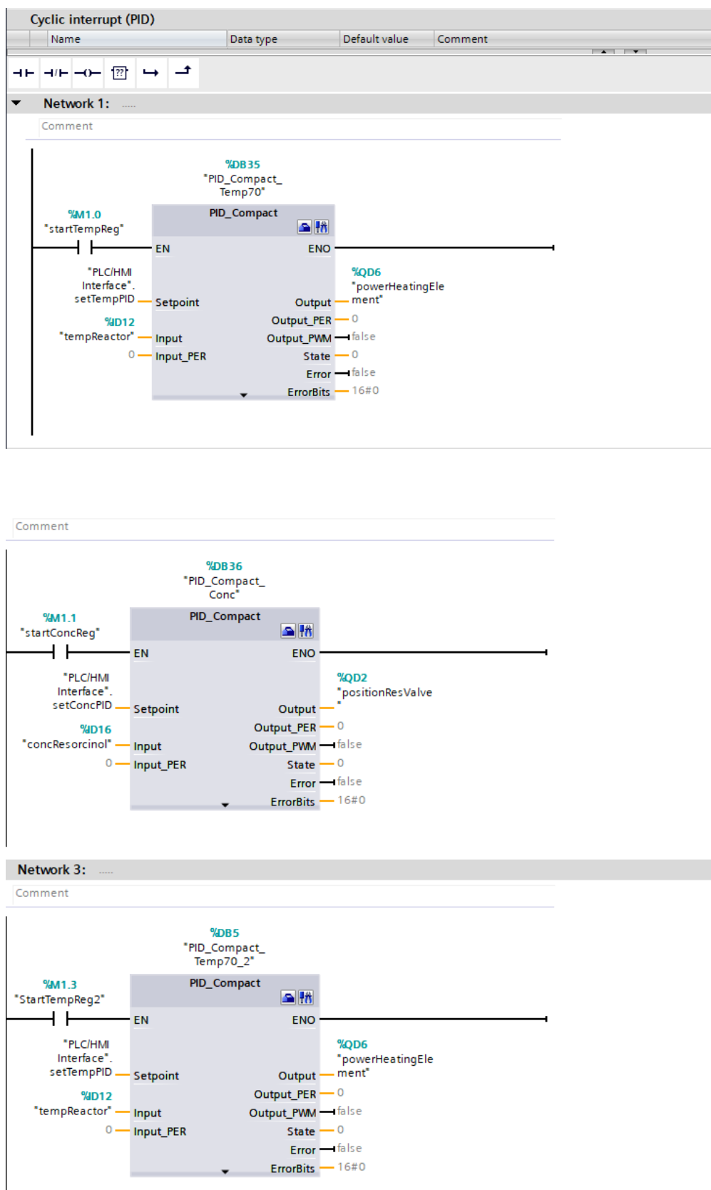
Figure D.0.3: Cyclic interrupt (PID)
