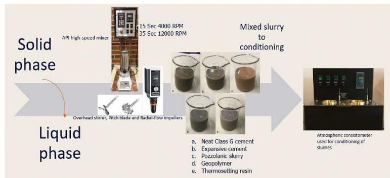
Fig. 2. Slurry sample preparation for laboratory tests.
