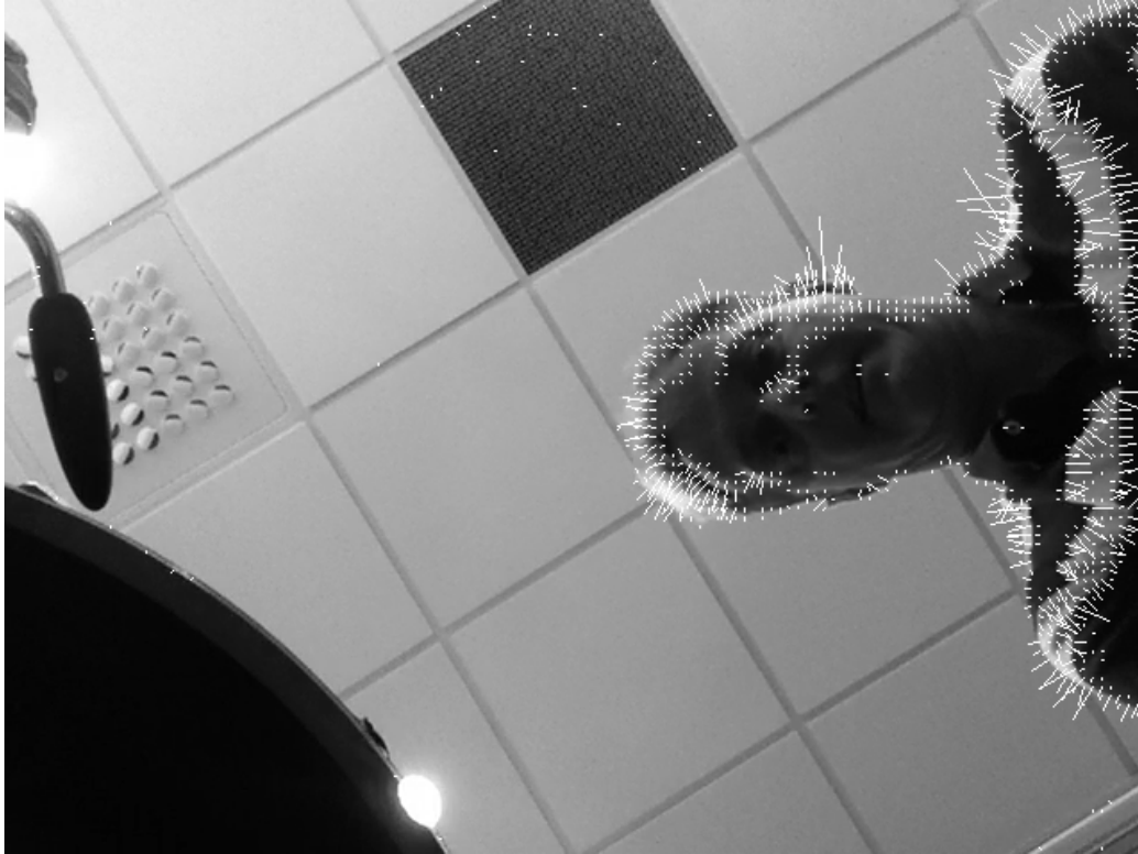
Figure 3.6: Optical flow motion vectors.
