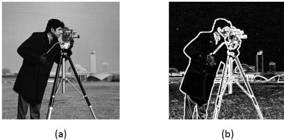
Figure 10 Image with and without Sobel filter
