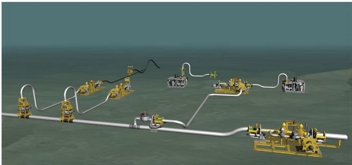
Figure 3-5 Spool's connected to subsea structures (PLEM, X-tree and Tee' - FMC Technologies)
