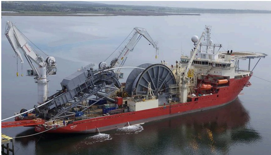
Figure 3.4 Apache II reeling on-board a pipeline [19].
