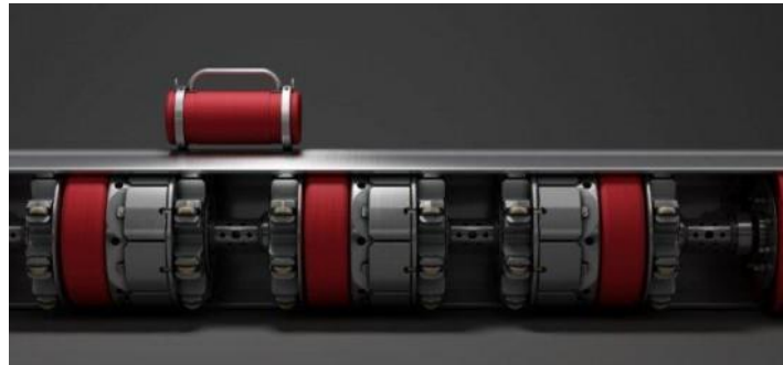
Figure 2.3-6: Smart pig with tracer [14]
