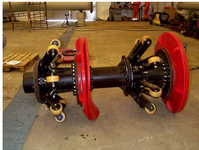
Figure 2.3-9: Multi diameter pig, special cup with contoured areas [16]
