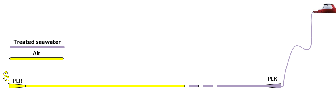
Figure 4.1-1: Flooding and cleaning
