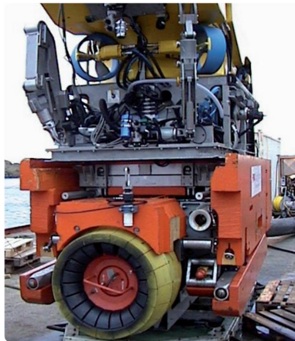
Figure 3.8-7: ROVCON collet connection tool [42]
