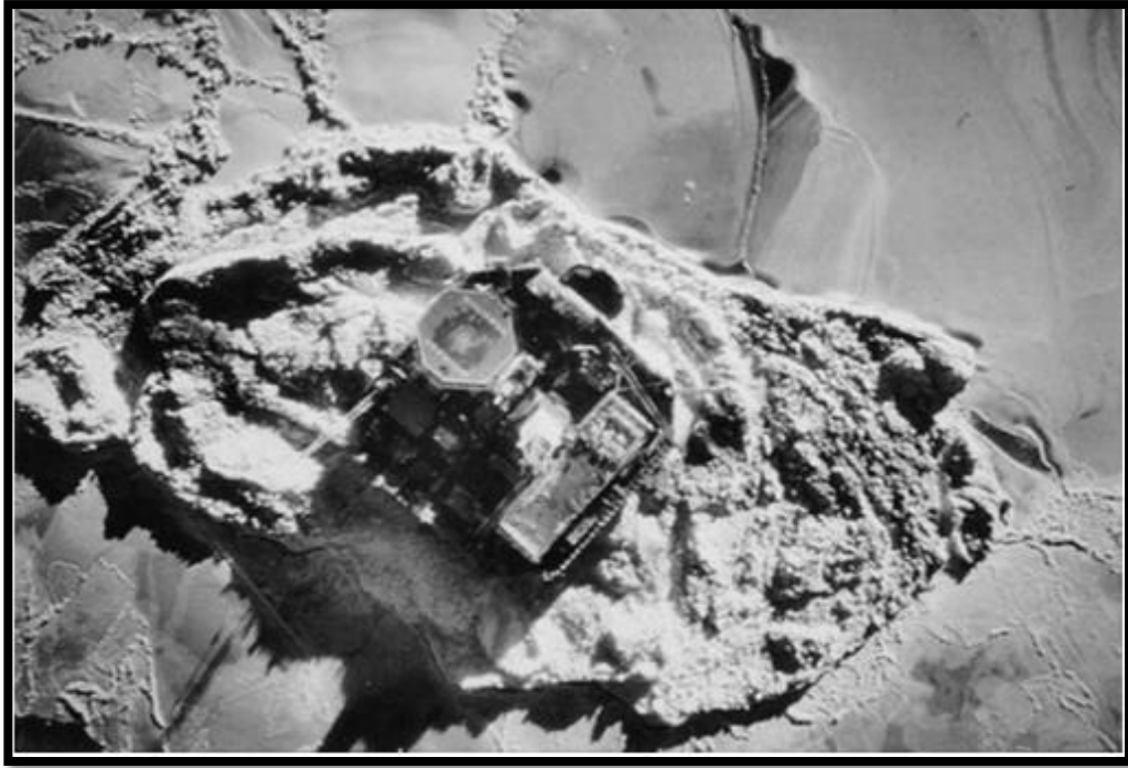
Figure 15: Grounded rubble field surrounding the Molikpaq at the Amauligak F-24 site (Timco et. al., 2006)
