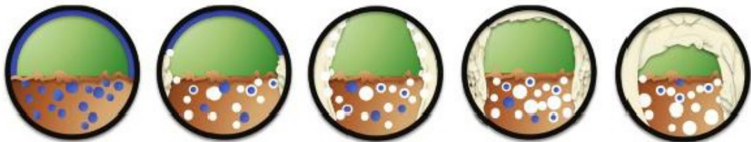
Figure 7. Hydrate deposition of the pipe wall [33]
