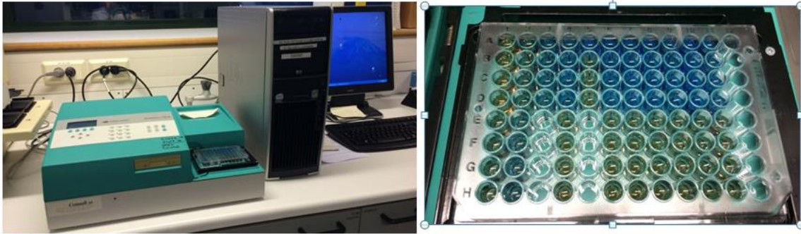
Figure 12. Spectroscope, using Bradford method for finding the protein concentration
