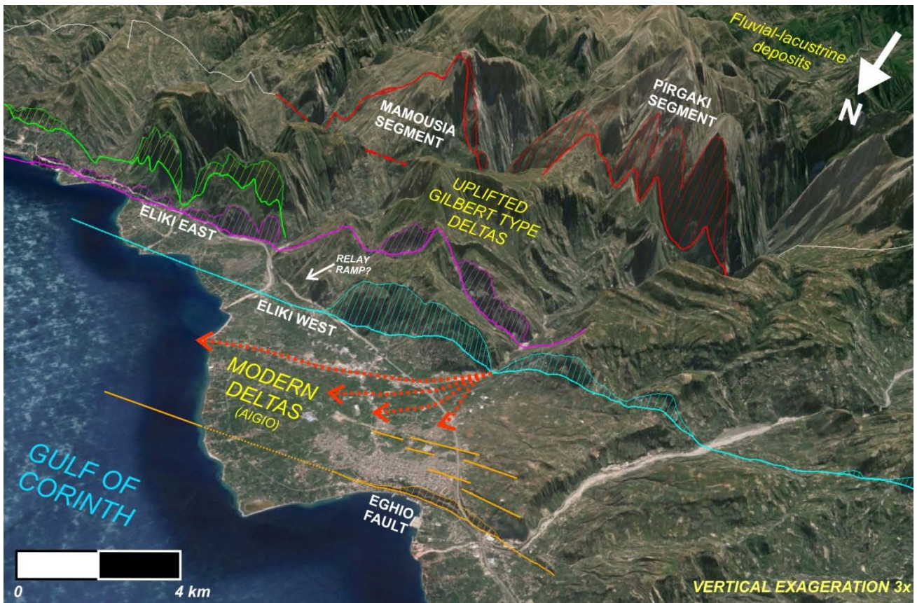
Figure 33 - Google Earth satellite image integrated with DEM (Google, 2015b) showing a sketch of relations between mapped structural, lithological and geomorphological features. Main points to be highlighted are: (i) Structural interpretation derived from field data with generalized fault footwall exposure; (ii) Simplified lithological compartmentalization with dominant units for each region; (iii) Relay ramp influence on development on sedimentation paths shown as red dotted arrows.
