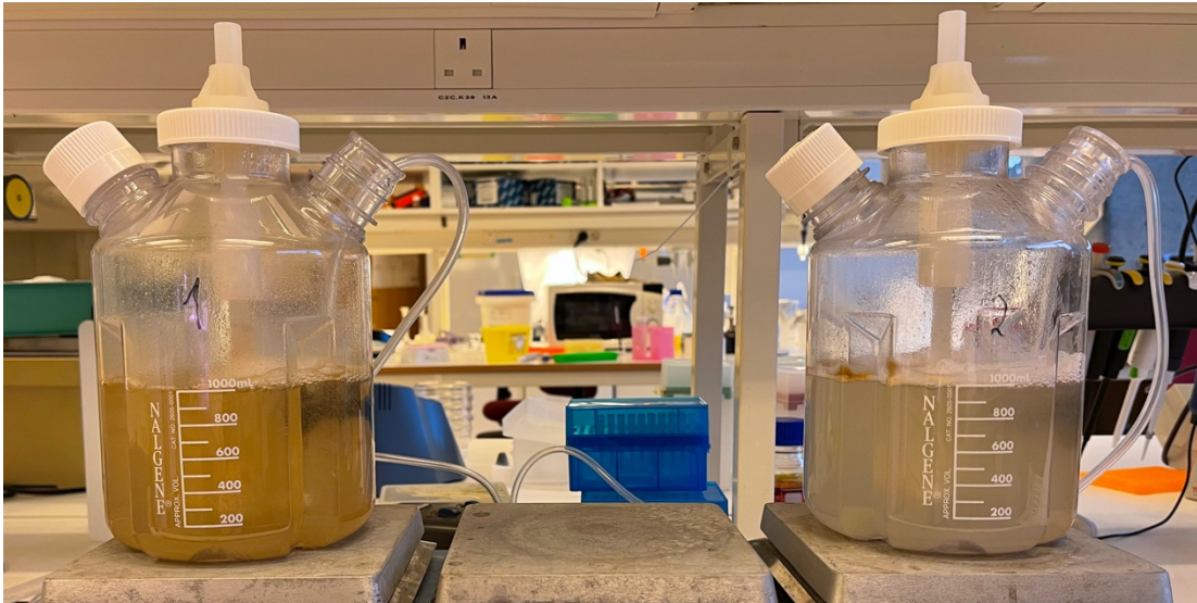
Figure 14. Reactor 1 on the left, and reactor 2 on the right side. Flocs and forming of biofilms in reactor 2 can be seen. The water in reactor 2 became clearer over time.
