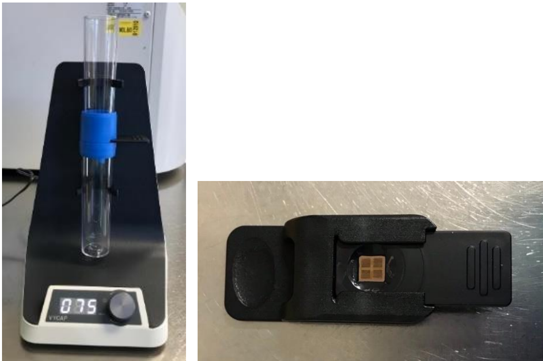
Figure 5. VYCAP Equipment. VYCAP pump unit (left) and microsieve (right).
