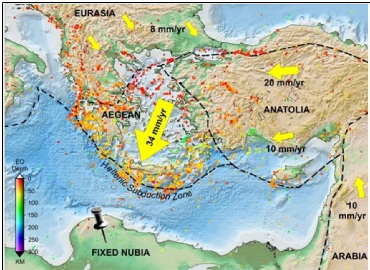
Figure 2-1: Plate tectonics in eastern Mediterranean. Arrows showing plate movement relative to a fixed Nubia (African plate) (Apel et al., 2007).
