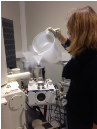
Figure 6: Cryo-SEM; regularly refilling the dewars with liquid nitrogen
