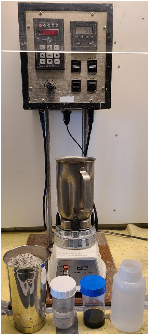
Figure 1: Commercial blender setup with ingredients from left to right; Precursor, Retarder, Superplasticizer and Activator
