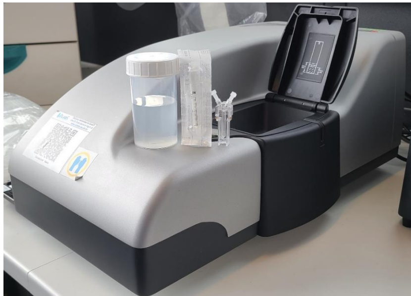
Figure 6: Zetasizer together with a sample, sterile syringe and DTS1070 container
