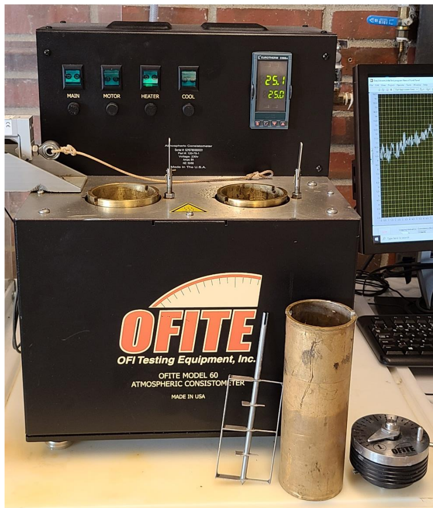
Figure 2: Ofite Model 60 Atmospheric Consistometer
