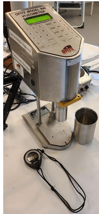
Figure 3: Ofite Model 900 Viscometer, stopwatch and measuring cup.
