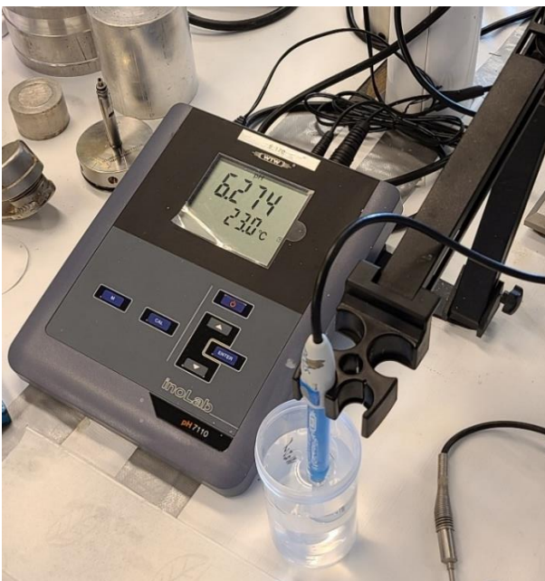
Figure 4: inoLab pH 7110 used for pH measurements
