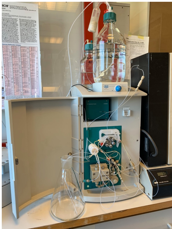
Figure 4. Ion chromatography setup for analysis of cations with eluent (top flask), conductivity detector (green box on shelf) and column heater containing column (right black box) at NIBIO Særheim.
