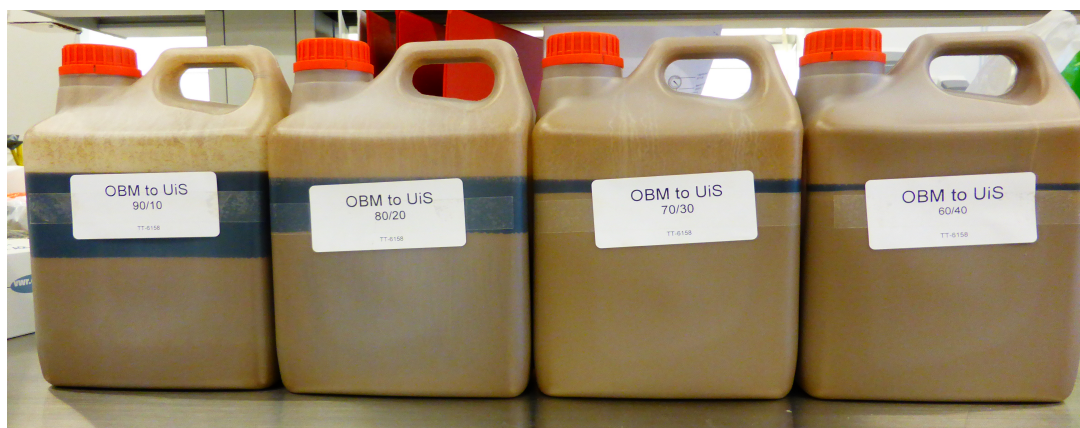
Figure 2: Illustration of the 60/40, 70/30, 80/20 and 90/10 oil based mud systems.
