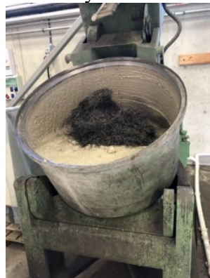
Figure 3. 2: Concrete mixer used during the experiment.
