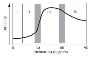
Figure 7 difficulty of efficient hole cleaning for different inclinations (Amanna, B et al 2016)
