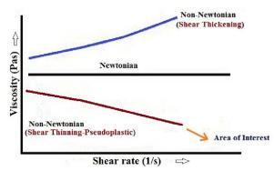
Figure 1 Behavior of different fluids when shear forces are applied, Baek, W 2013)
