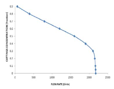
Hydraulic optimization is another factor in achieving efficient hole cleaning. Determining the optimal pressure drop across the bit, optimum jet impact force at the bit could be used to optimize the flow rate for hole cleaning. This information could be used to find the correct pumping pressure to achieve the optimized flow rate in the well. Finding the optimal flow rate is essential due to it together with drill pipe rotation
