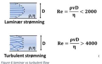
The flow regime around the drill string plays an important role in effective hole cleaning. Flow regimes are often characterized as either laminar or turbulent. Laminar flow occurs when the fluid flow in parallel layers with no disruption between them and Reynolds number for laminar flow should be below 2000. The Reynold number gives
