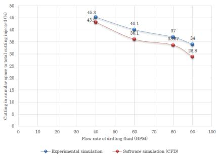
The computer then used the equation 23 to estimate cutting in the annular space for different flow rates. Software data was then compared to experimental data. Simulated cutting concentration changed in accordance with what they observed during experiments and indicates simulations
