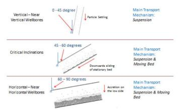
Figure 3 Transport of cuttings for different inclinations (Tomren et al 1986)
