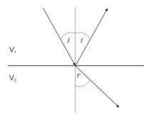
Figure 4 Acoustic waves refraction trough 2 mediums
