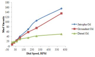
it is more shear thickening than diesel, commonly considered an undesirable trait for drilling fluids This was demonstrated in an experiment and the results can be observed in Figure 9. (Wardana, ING 2010 and Fadairo, AS et al 2013, Anawe, P et al 2014 and Abduo, MI et al 2016))
