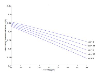
Figure 6-hole cleaning with 60 degrees inclination under different flow rates (Ammana et al 2016).
