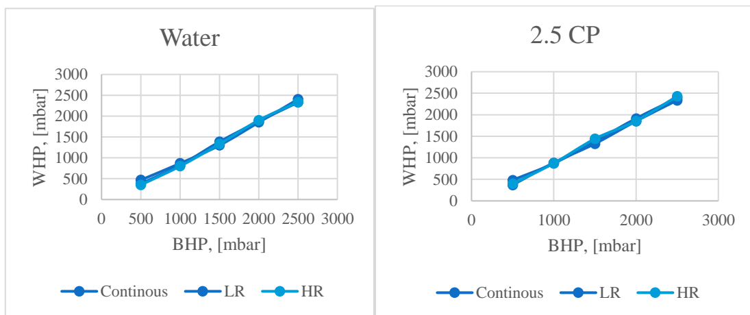
Figure 4.2.7: Water as fluid in the wellbore with BHP vs WHP, b, 2,5 CP as fluid in the wellbore with BHP vs WHP
