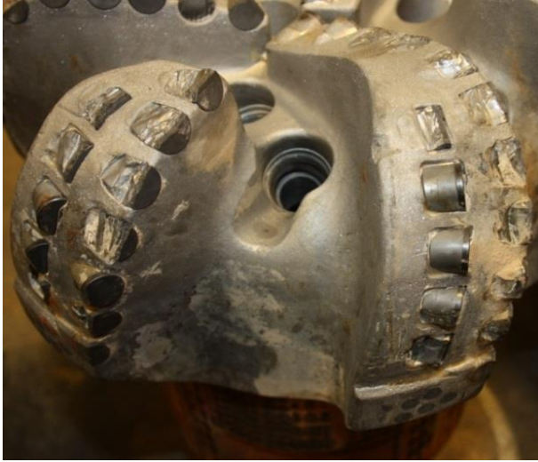
Figure 27. Bit dull-picture, MMD65DH, well #4 [12]
