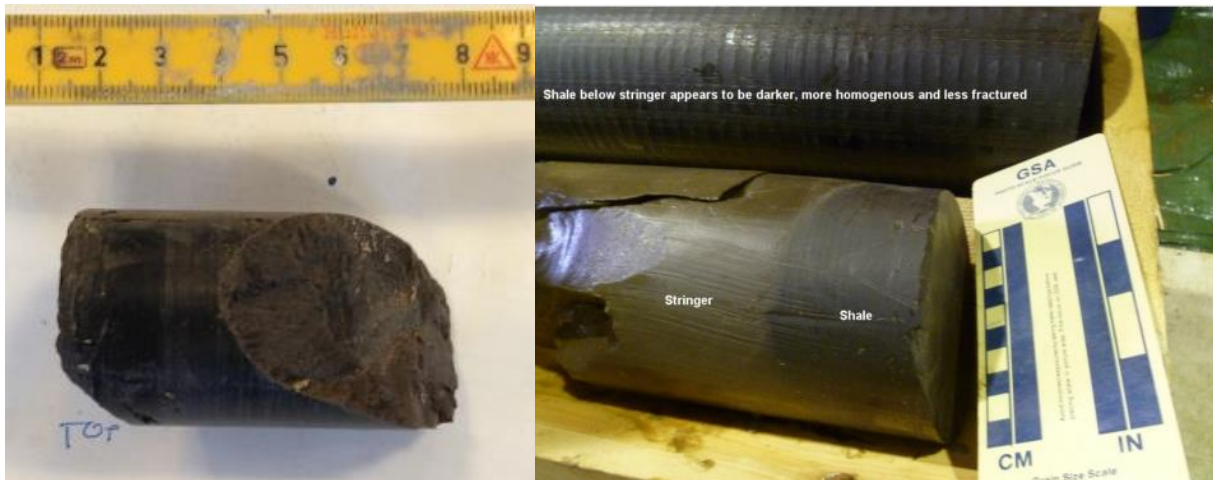
Figure 3. Core samples of shale (left) and limestone stringer (right) [8]
