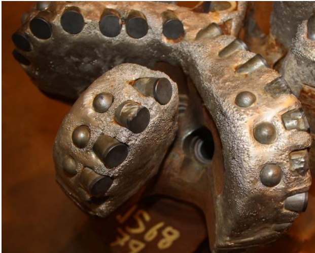
Figure 23. Bit dull-picture, SFG75, well #1 [12]
