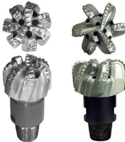
Figure 5. Matrix-body (left) and Steel-body (right) PDC bits [1]
