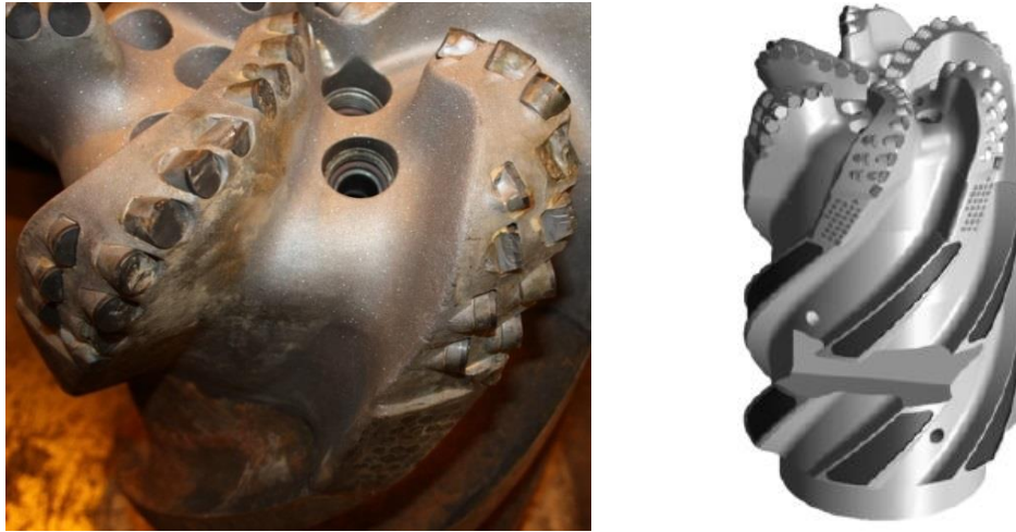
Figure 25. Bit dull-picture, FXG65D, well #2 [12]
