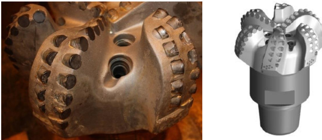
Figure 26. Bit dull-picture, MMD65DH, well #3 [12]
