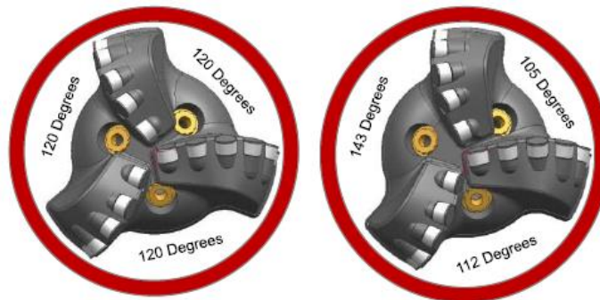
Figure 13. Symmetric (left) and Asymmetric (right) blades layout [1]
