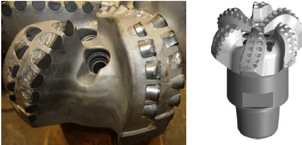
Figure 29. Bit dull-picture, MMD65DH, well #5 [12]
