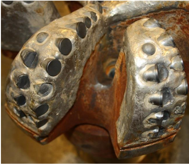
Figure 44. Bit dull-picture, SFD65D, used on Ekofisk overburden [12]
