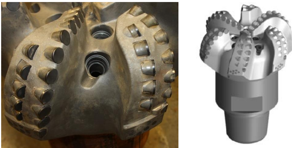
Figure 30. Bit dull-picture, MMD65DH, well #6 [12]
