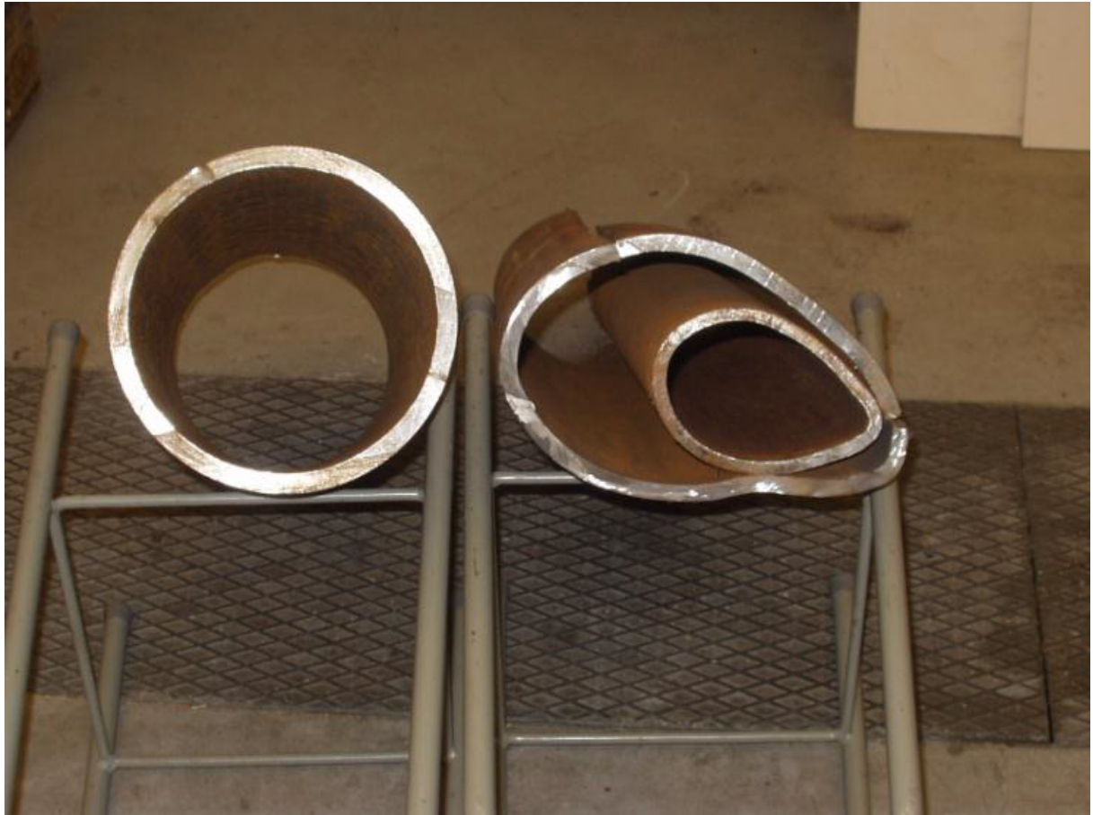
Figure 37: Collapsed casing and tubing from a North Sea well [Torbergsen et al., 2012]
