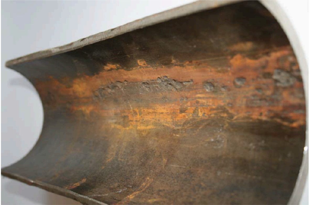
Figure 4: Local corrosion of L80 13Cr tubing [Bellarby, 2009]
