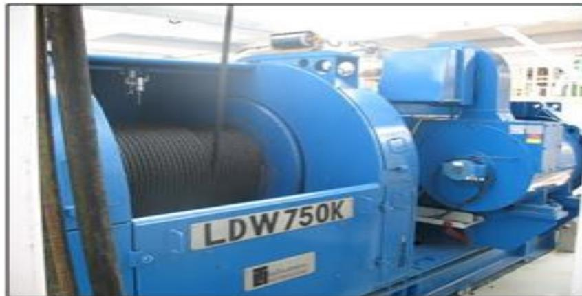
**Figure 11: shows a conventional draw work hoisting system by courtesy of directional drilling technology blog [6]**
