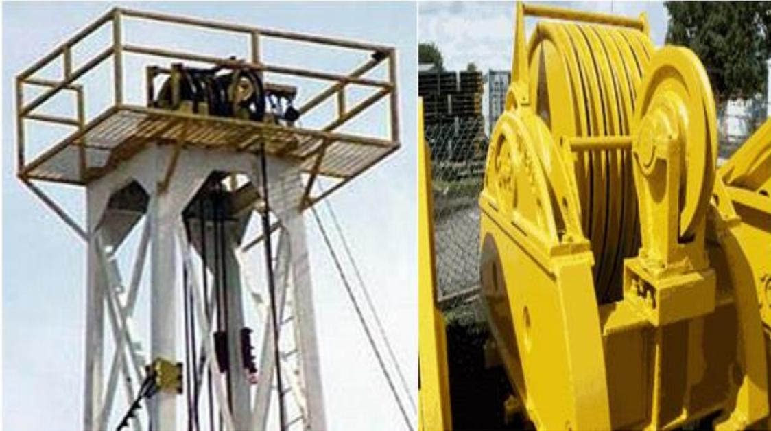
Figure 9: shows a the crown block sheave arrangements, to the left is the zoomed-out view and to the right is the zoomed-in view by courtesy of directional drilling technology blog [6]
