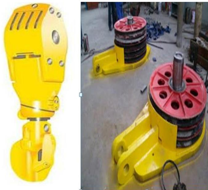
Figure 10: shows the travelling block. To the left is the travelling block sheave in its protective housing while to the right shows an opened protective travelling block housing by courtesy of directional drilling technology blog [6]
