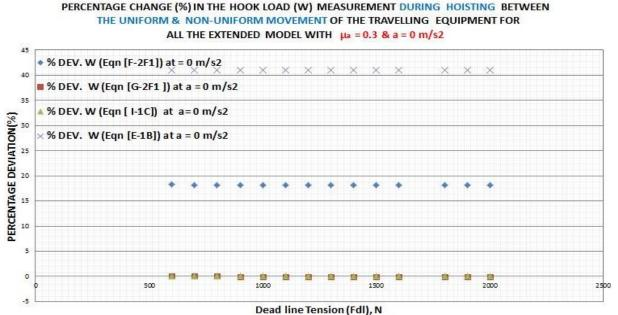
Figure 67: Shows the percentage deviation of all the extended hook load measurement during hoisting with uniform movement of the travelling equipment from the sum of the tensions in the supporting lines also during uniform movement of the travelling equipment based on the extended Cayeux et al hook load prediction for  $e \approx 0.83$  ( $\mu_a = 0.3$ ) & a = 0 m/s<sup>2</sup>
