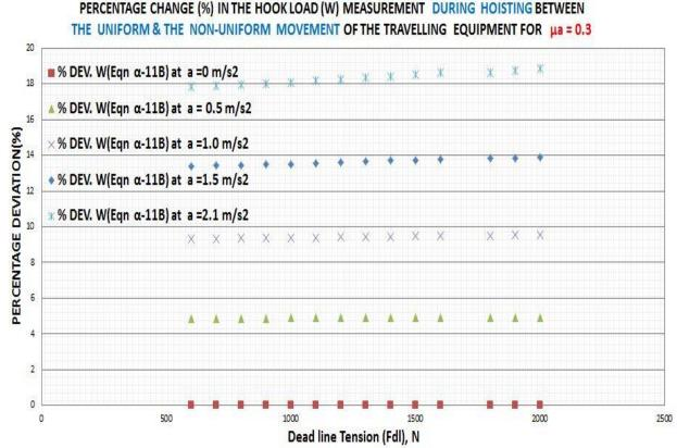
Figure 44: Shows the percentage deviation of the extended Cayeux et al hook load value during hoisting with non-uniform movement of the travelling equipment from the sum of the tensions in the supporting lines during uniform movement also based on the extended Cayeux et al hook load prediction model for  $\mu_a = 0.3$
