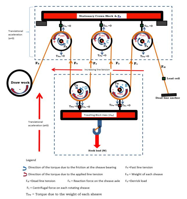
Figure 27: The forces and torques on both the crown block and the travelling block sheaves during hoisting
