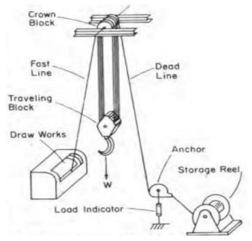
Figure 8: shows a conventional draw work hoisting system by courtesy of Bourgoyne et al 1986 [9]
