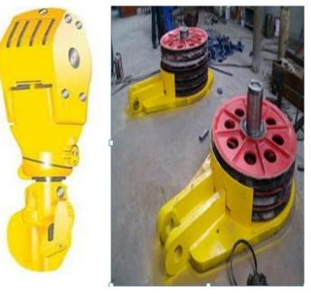
Figure 10: shows the travelling block. To the left is the travelling block sheave in its protective housing while to the right shows an opened protective travelling block housing by courtesy of directional drilling technology blog [6]
