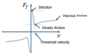
Figure 2: Schematic showing the transition from static coefficient of friction to dynamic coefficient of friction and vice-versa by courtesy of Cayeux et al [4]
