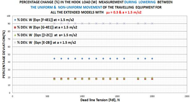
Figure 77: Shows the percentage deviation of all the extended hook load value during lowering with non-uniform movement of the travelling equipment from the sum of the tensions in the supporting during uniform movement based on the extended Cayeux et al hook load prediction model for  $e \approx 0.83$  ( $\mu_a = 0.3$ ) & a = 1.5 m/s<sup>2</sup>
