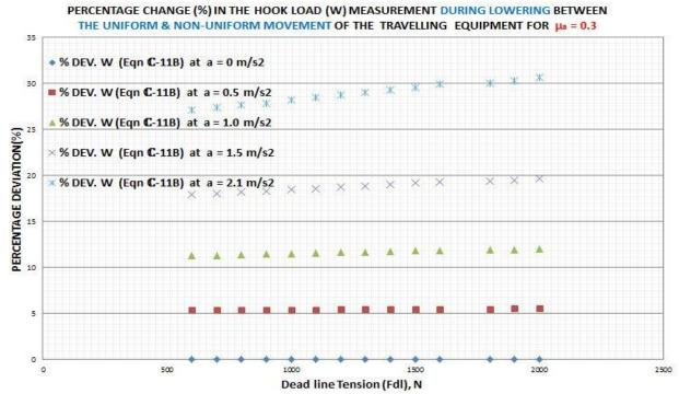
Figure 53: Shows the percentage deviation of the extended Cayeux et al hook load values during lowering with non-uniform movement of the travelling equipment from the sum of the tensions in the supporting lines during uniform movement also based on the extended Cayeux et al hook load prediction model for  $\mu_a = 0.3$
