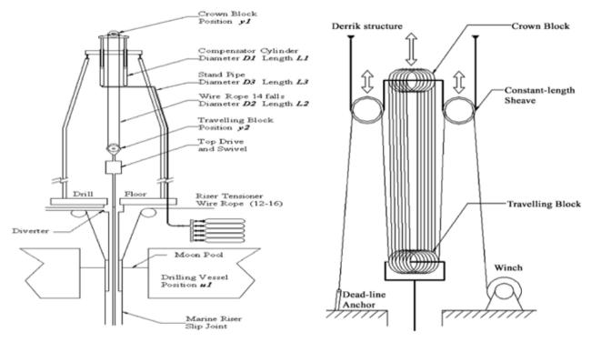
Figure 12: shows Passive heave compensation by courtesy of Hatleskog and Dunnigan (2007). To the left is the zoomed-out view of the Passive heave compensation while to the right is the zoomed-in view of the Passive heave compensation [7]
