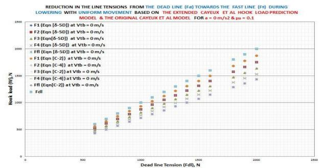
Figure 46: Shows the extended Cayeux et al hook load values during lowering with uniform movement of the travelling equipment for  $\mu_a = 0.1$
