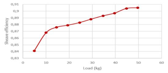
Figure 4: Shows variation in the sheave efficiency as a function of the applied load by courtesy of Cayeux et al [4]
