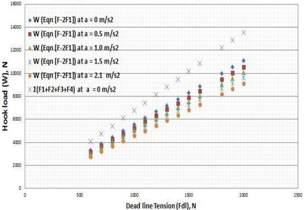
Figure 56: Shows the extended Luke and Juvkam hook load values during hoisting with non-uniform movement of the travelling equipment assuming constant sheave efficiency  $e \approx 0.818$  which corresponds to  $\mu_a = 0.3$
