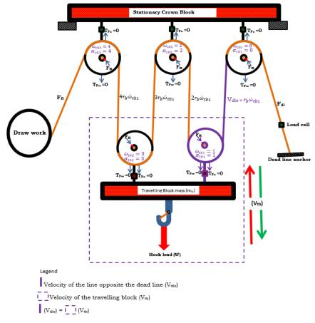
Figure 28: Shows the relationship between the travelling block velocity  $(V_{tb})$  and the angular velocity of the first sheave  $(\dot{\omega}_{tb1})$  in the travelling block connected by the line opposite the dead line
