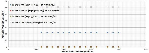
Figure 75: Shows the percentage deviation of all the extended hook load values during lowering with uniform movement of the travelling equipment from the sum of the tensions in the supporting lines during uniform movement based on the extended Cayeux et al hook load prediction model for  $e \approx 0.818$  ( $\mu_a = 0.3$ ) & a = 0 m/s<sup>2</sup>
