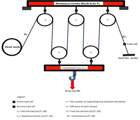
Figure 18: Show a block and tackle hoisting system and its constant sheave efficiency as proposed by Luke and Juvkam- Wold
