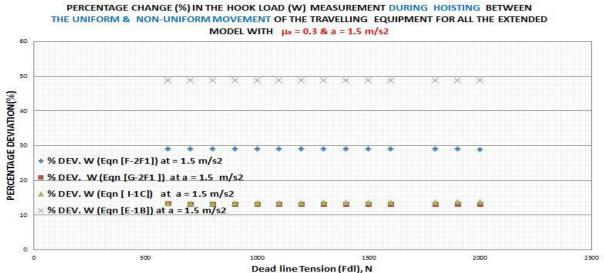
Figure 69: Shows the percentage deviation of all the extended hook load values during hoisting with non-uniform movement of the travelling equipment from the sum of the tensions in the supporting lines during uniform movement of the travelling equipment based on the extended Cayeux et al hook load prediction for  $e \approx 0.83$  ( $\mu_a = 0.3$ ) & a = 1.5 m/s<sup>2</sup>
