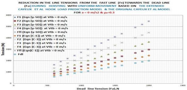
Figure 39: Shows the tensions in the lines during imperfect transmission of the line tension  $(\mu_a = 0.3)$
