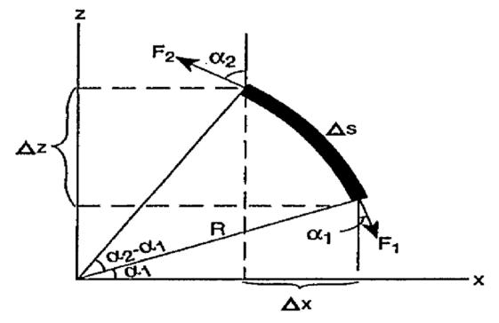
Figure 16: Shows the torque and drag in a drop-off section by courtesy of Aadnøy and Andersen [10]
