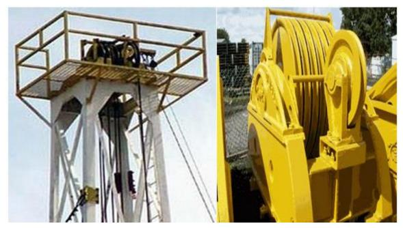
Figure 9: shows a the crown block sheave arrangements, to the left is the zoomed-out view and to the right is the zoomed-in view by courtesy of directional drilling technology blog [6]
