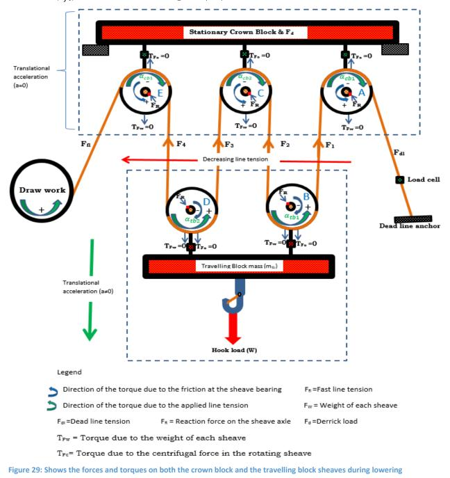
Considering the dead line sheave (sheave A) in the crown block, the net the torque is given by Eqn  $[H-3C_1]$  as (see Appendix C for derivation)
