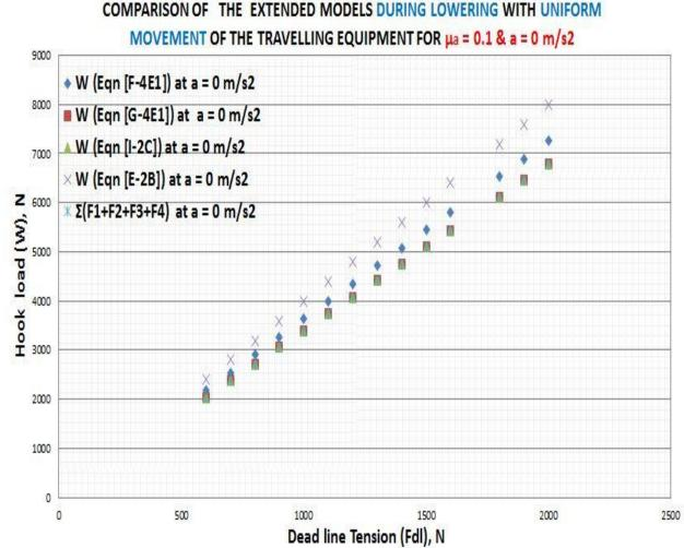
Figure 72: Shows the comparison of all the extended hook load prediction models during lowering with uniform movement of the travelling equipment and the sum of the tensions in the supporting lines also during uniform movement based on the extended Cayeux et al hook load prediction model for  $e \approx 0.94$  ( $\mu_a = 0.1$ ) & a = 0 m/s<sup>2</sup>
