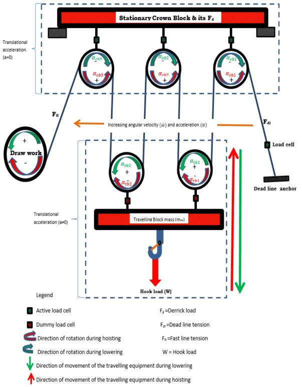
Figure 24: shows the direction of rotation of the sheave for both the crown block sheaves and the travelling block sheaves during hoisting and lowering
