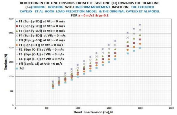
Figure 37: Shows the tensions in the lines during slightly imperfect transmission of the line tension ( $\mu_a = 0.1$ )
