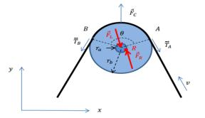
Figure 19: Shows the forces on the crown block sheave by courtesy of Cayeux et al [4]
