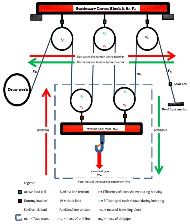
Figure 20: Shows the total mass of the travelling equipment and the direction of the resultant force during either hoisting or lowering
