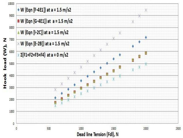
Figure 76: Shows the comparison of all the extended hook load prediction models during lowering with non-uniform movement of the traveling equipment and the sum of the tensions in the supporting also during uniform movement based on the extended Cayeux et al hook load prediction model for  $e \approx 0.818$  ( $\mu_a = 0.3$ ) & a = 1.5 m/s<sup>2</sup>
