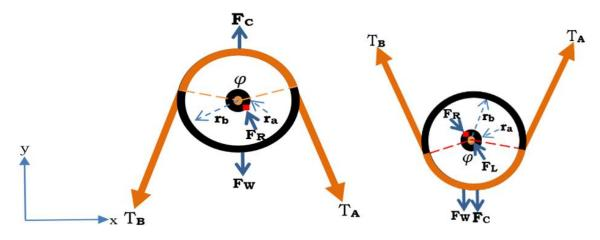
Figure 26: Shows the applied  $load(F_L)$  and its corresponding reaction force  $(F_R)$  on a crown block and a travelling block sheaves respectively
