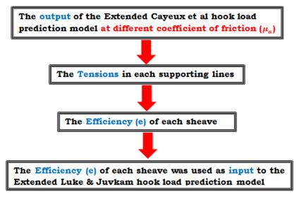
Figure 30: Schematic illustrating how the output of the extended Cayeux et al hook load prediction model was used as input to the extended Luke and Juvkam hook load prediction model
