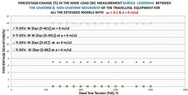
Figure 73: Shows the percentage deviation of all the extended hook load measurement during lowering with uniform movement of the travelling equipment from the sum of the tensions in the supporting lines during uniform movement based on the extended Cayeux et al hook load prediction model for  $e \approx 0.94$  ( $\mu_a = 0.1$ ) & a = 0 m/s<sup>2</sup>
