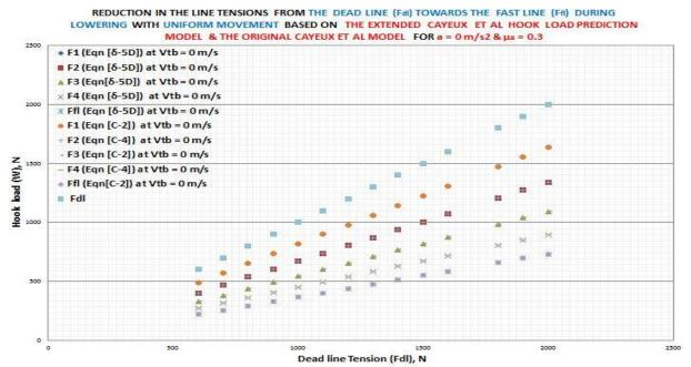
Figure 48: Shows the extended Cayeux et al hook load value during lowering with uniform movement of the travelling equipment for  $\mu_a = 0.3$
