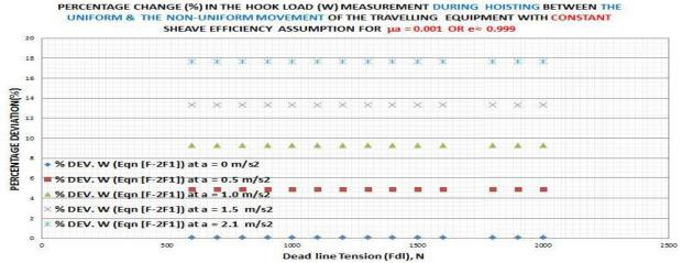
Figure 55: Shows the percentage deviation of the extended Luke and Juvkam hook load values during hoisting with non-uniform movement of the travelling equipment from the sum of the tensions in the supporting lines during uniform movement based on the extended Cayeux et al hook load prediction model for  $e \approx 1$  ( $\mu_a = 0.001$ )
