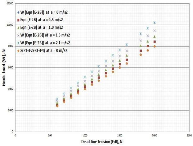
Figure 33: Shows the extended Industry accepted hook load values during lowering with nonuniform movement of the travelling equipment
