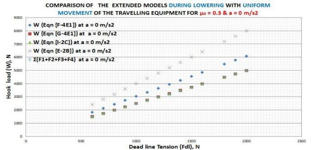
Figure 74: Shows the comparison of all the extended hook load prediction models during lowering with uniform movement of the traveling equipment and the sum of the tensions in the supporting lines also during uniform movement based on the extended Cayeux et al hook load prediction model for  $e \approx 0.83$  ( $\mu_a = 0.3$ ) & a = 0 m/s<sup>2</sup>
