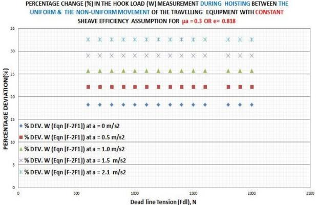
Figure 57: Shows the percentage deviation of the extended Luke and Juvkam hook load values during hoisting with non-uniform movement of the travelling equipment from the sum of the tensions in the supporting lines during uniform movement based on the extended Cayeux et al hook load prediction model for  $e \approx 0.818$  ( $\mu_a = 0.3$ )
