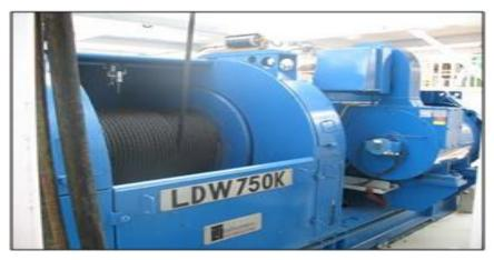
Figure 11: shows a conventional draw work hoisting system by courtesy of directional drilling technology blog [6]
