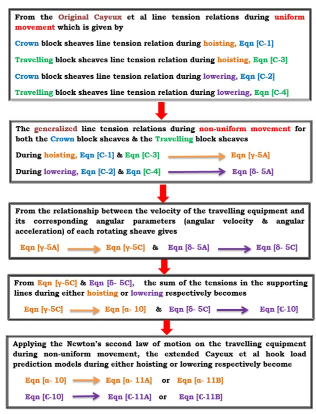
Figure 78: Schematic illustrating how the extended Cayeux et al hook load prediction model during non-uniform movement of the travelling block was obtained
