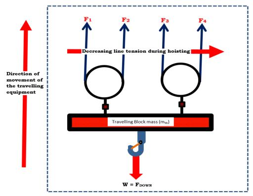
Figure 22: Shows the net force on the travelling equipment during hoisting
