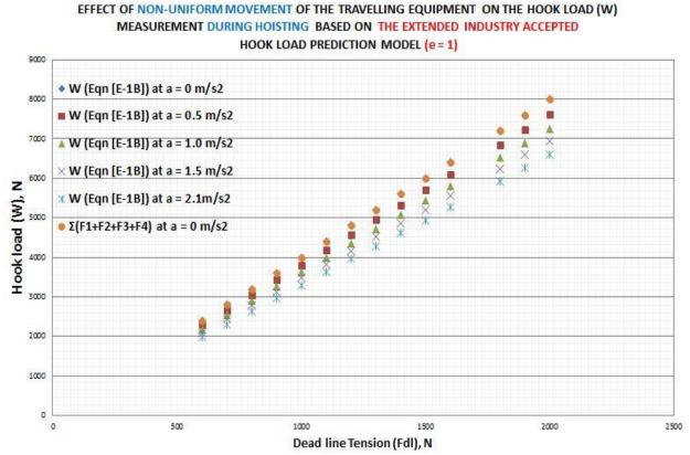
Figure 31: Shows the extended Industry accepted hook load value during hoisting with nonuniform movement of the travelling equipment
