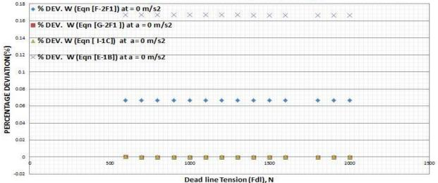
Figure 63: Shows the percentage deviation of all the extended hook load values during hoisting with uniform movement of the travelling equipment from the sum of the tensions in the supporting lines also during uniform movement based on the extended Cayeux et al hook load prediction model for  $e \approx 1 \ (\mu_a = 0.001)$  & a = 0 m/s2
