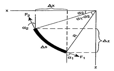
Figure 15: Shows the torque and drag in a build-up section by courtesy of Aadnøy and Andersen [10]
