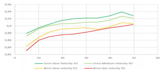
Figure 5: Shows variation in the average sheave efficiency during hoisting and lowering for different applied loads, different elasticity of the drill-line and at different speed of the travelling equipment by courtesy of Cayeux et al [4]
