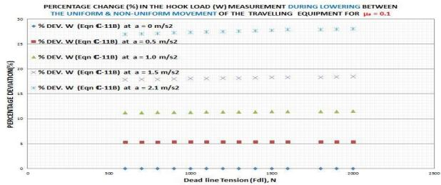
Figure 51: Shows the percentage deviation of the extended Cayeux et al hook load values during lowering with non-uniform movement of the travelling equipment from the sum of the tensions in the supporting lines during uniform movement also based on the extended Cayeux et al hook load prediction model for  $\mu_a = 0.1$
