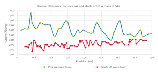
Figure 3: Shows the variation in sheave efficiency as a function of block position and direction of movement of the travelling equipment (hoisting or lowering) by courtesy of Cayeux et al [4]
