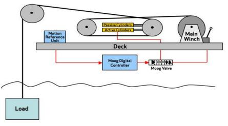
Figure 13: Is a schematic of a Rotative Active Heave Compensation (RAHC) by kind courtesy of offshoreteknikk [8]
