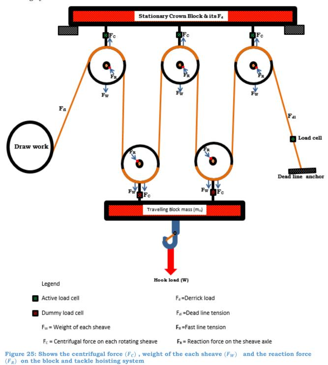
Based on Coulomb friction  $model(\mu_a)$ , the magnitude of the torque due to the friction at the sheave axle is given by  $\|\overrightarrow{M_f}\| = \mu_a r_a \|\overrightarrow{F_R}\|$
