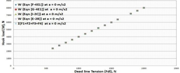
Figure 70: Shows the comparison of all the extended hook load prediction models during lowering with uniform movement of the traveling equipment and the sum of the tensions in the supporting lines also under uniform movement based on the extended Cayeux et al hook load prediction model
