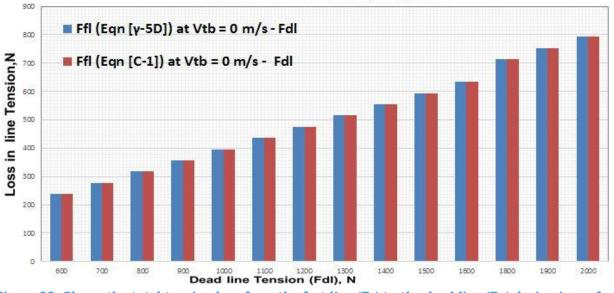
Figure 38: Shows the total tension loss from the fast line (Ffi) to the dead line (Fdi) during imperfect transmission of the line tension ( $\mu_a = 0.1$ )
