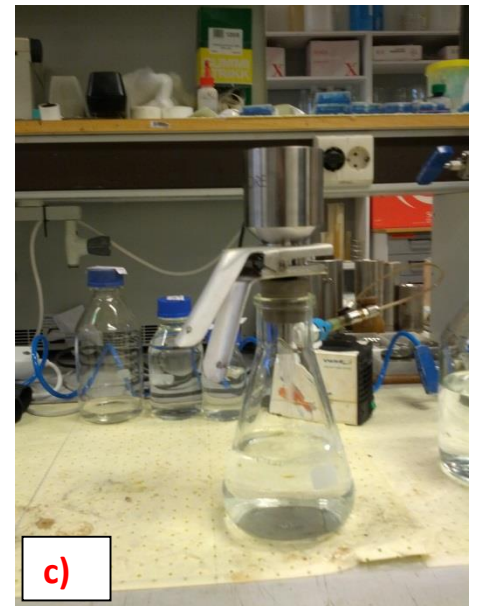
Figure 3.1 c) Filtrate-apparatus from Millipore used to filtrate the brine. A 0.65 µm filter used consistently for all the brine prepared.
