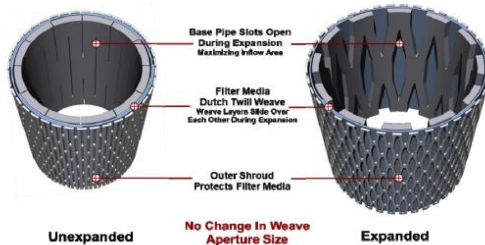
Figure 7 Expandable sand screens construction [12]
