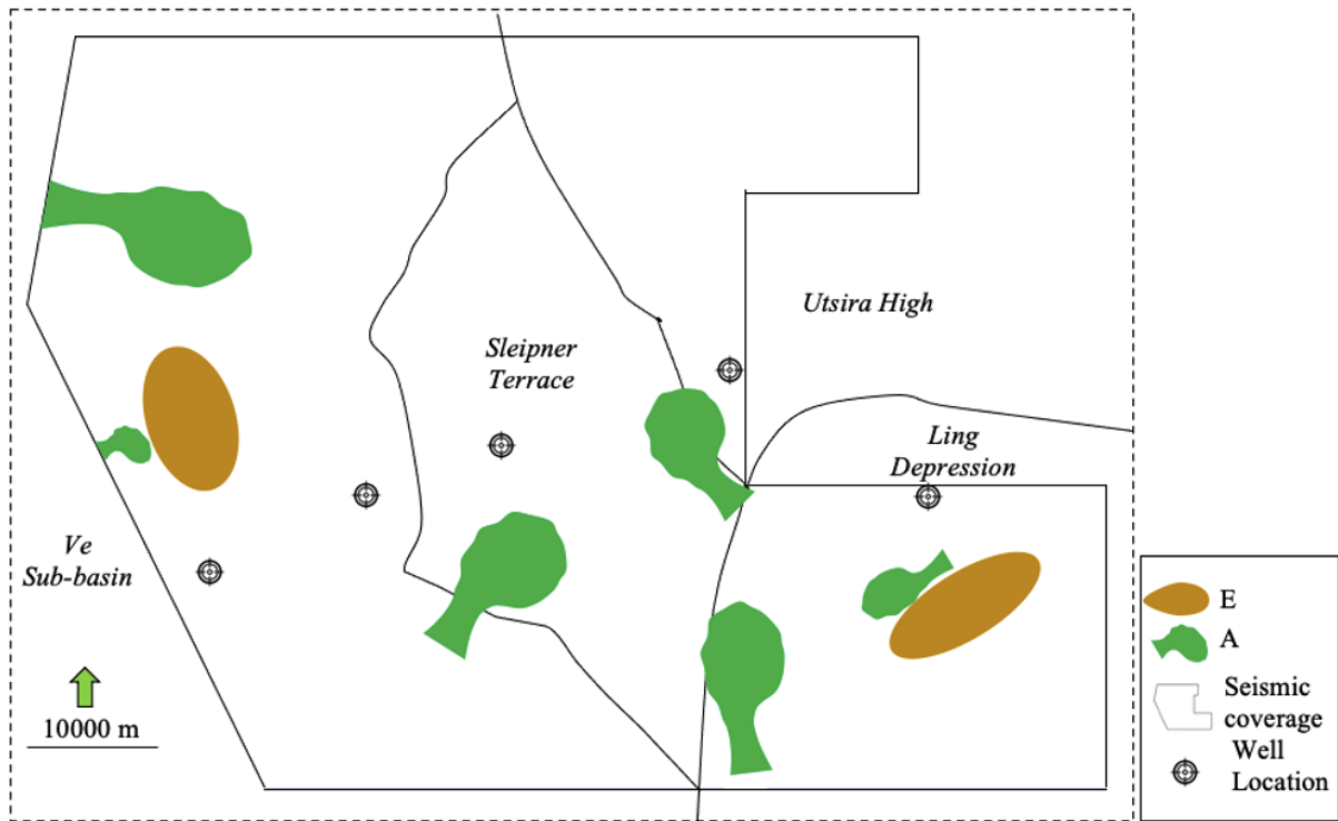
Figure 37: (Utsira Formation) seismic facies map showing facies A: Submarine channel and E: Mud diapir. The white parts within the seismic coverage are interpreted as the background sediments.
