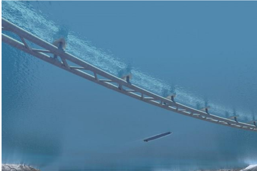
Figure 1-4: Submerged floating tunnel illustration [6]
