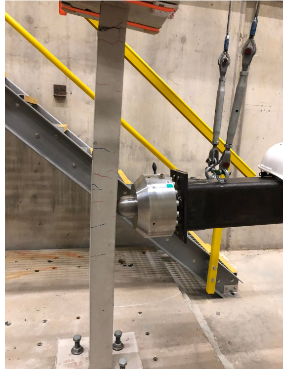
Figure 6.30. Deformation of Specimen10
