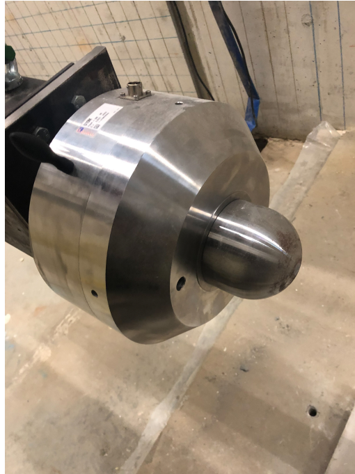
Figure 5.5. 500 kN Load Cell mounted with a steel tip on the end of the pendulum
