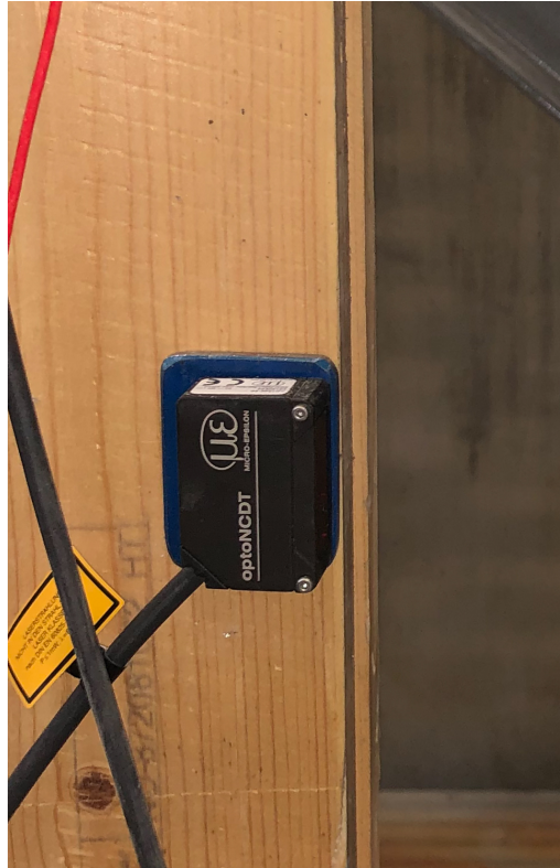
Figure 5.4. Laser displacement equipment used
