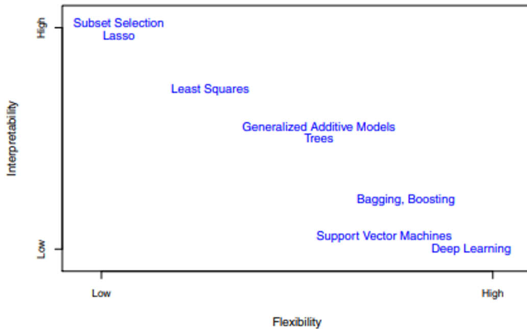
Figure 3.2: A representation of the tradeoff between flexibility and interpretability for the methods used in this study showing that generally if the method flexibility increases, its interpretability decreases[14]
