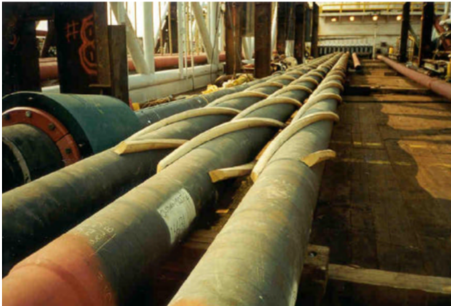
Figure 2.7: VIV suppression strakes [15]
