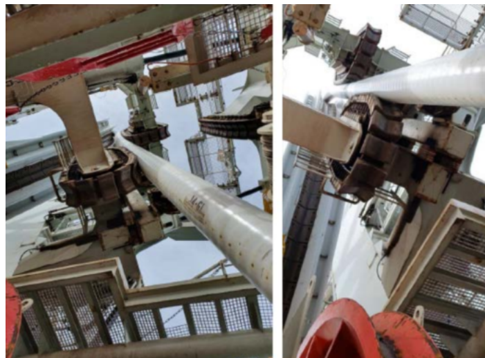
Figure 6.3: Straightener tracks configuration for straight pipe (left) and under-straightened residual curvature section (right) [31]
