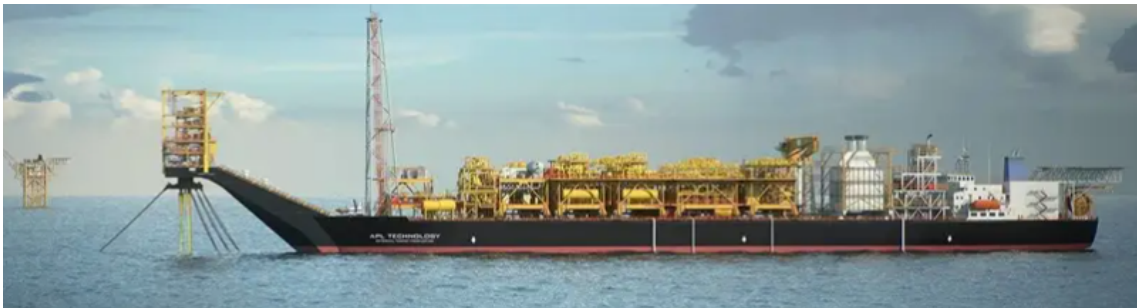
Figure 4.3: External turret on an FPSO [29]
