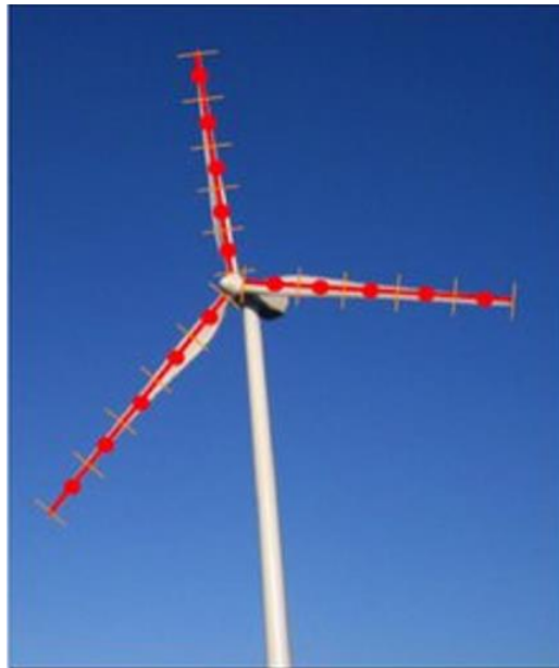
Figure 2-6 The discretization of the blades into the lines with each section representing the force [32]
