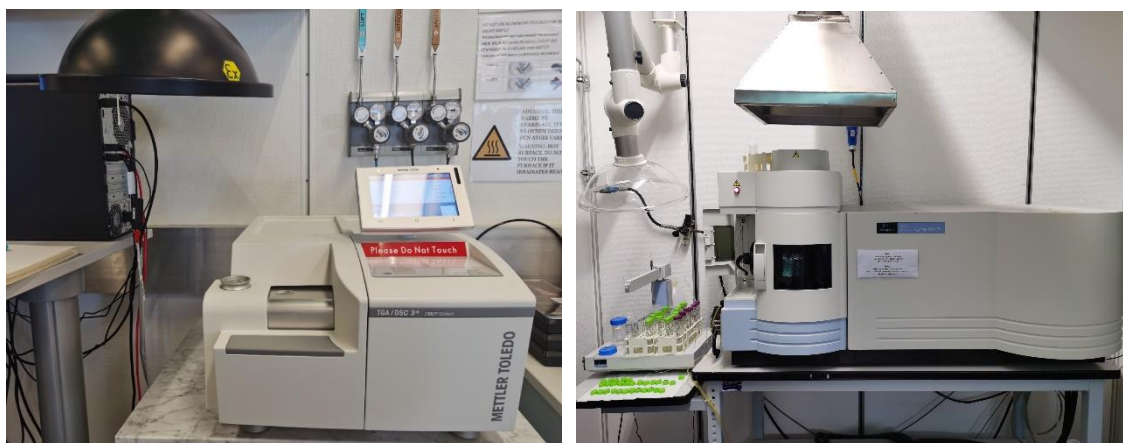
Figure 7. TGA/DSC 3+ (left) for TGA test and Optical Emission Spectrometer Optima 4300 DV (right) for ICP test.
