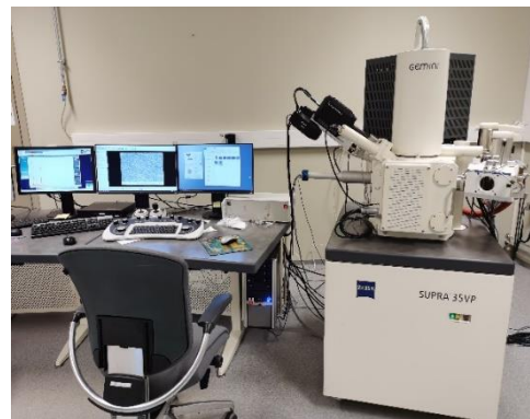
Figure 8. EM ACE600 (left) for coating rock samples with copper layer and SUPRA-35VP (right) for SEM & EDS analysis.
