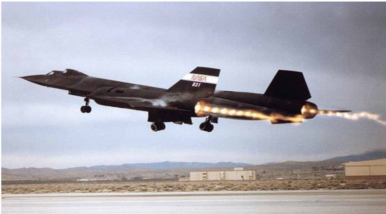
Figure 2. A series of Mach disks in the exhaust plume of jet engine (Bayeh, 2009).
