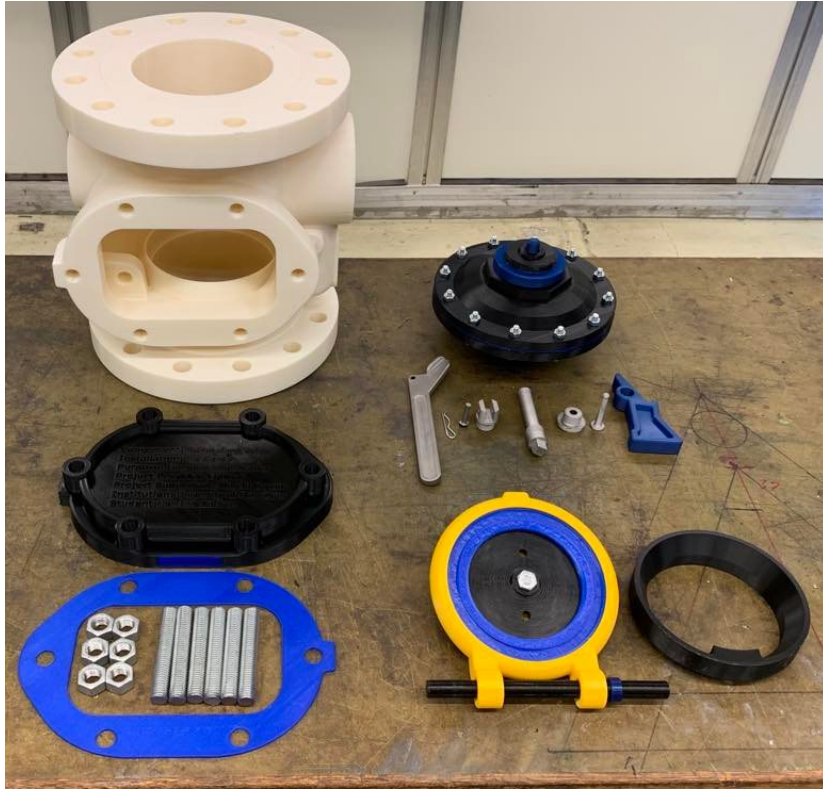
Figure 78: 3D-printed components of the reference valve
