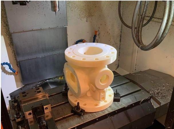
Figure 39: 3D printed reference valve body mounted in the MAZAK CNC machine
