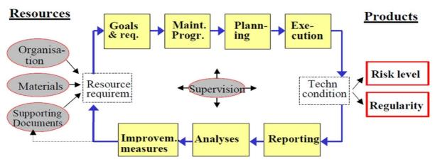
Figure 13 Maintenance management loop developed by the Norwegian Petroleum Directorate [31]
