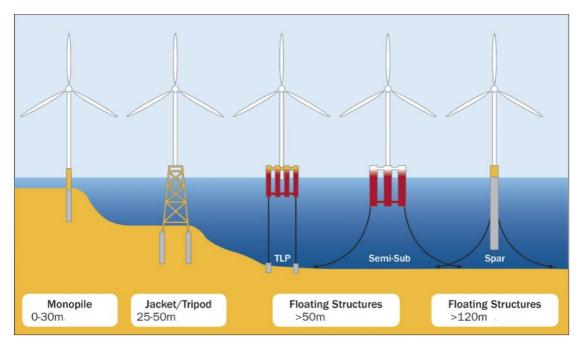
Figure 5: An overview of five of the most common foundations, two bottom-fixed and three floatings [23]
