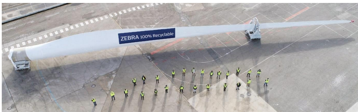
Figure 4.1: The first prototype of the 100% recyclable ZEBRA blade made by LM Wind Power. Photo credit ZEBRA consortium (GE, 2022).
