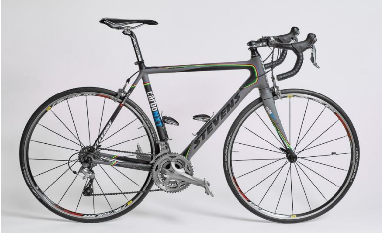
Figure B.6: Bicycle made with recovered carbon fibres from carboNXT. Photo by carboNXT (carboNXT, n.d.).
