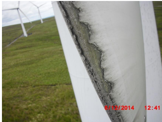
Figure 2.2: Typical blade damage from leading edge erosion (Belzona Polymerics Ltd., 2014).
