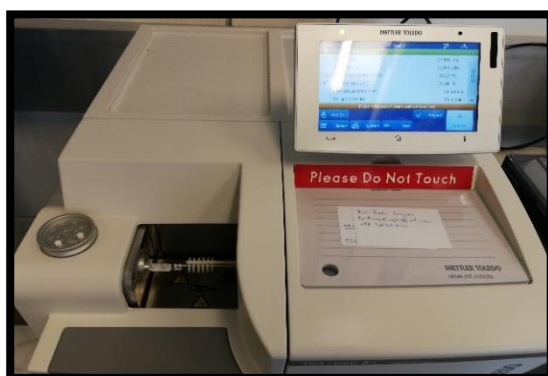
Figure 3.2. TGA instrument showing sample positions
