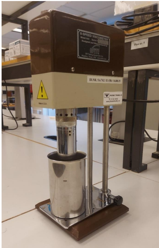
Figure 3.4: Viscometer OFITE Model 800
