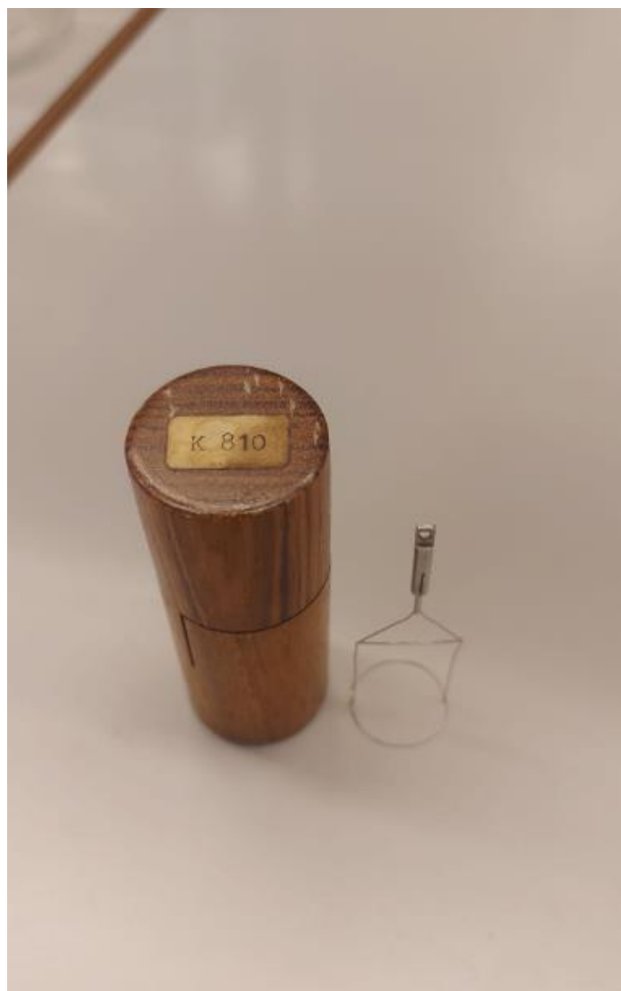
Figure 3.6: Ring K 810 Used for the measurement of Interfacial and Surface tension
