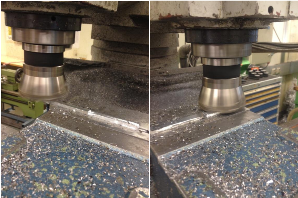
Figure 5-12, Figure 5-13 & Figure 5-14 Pre milled specimen and milling of specimen
