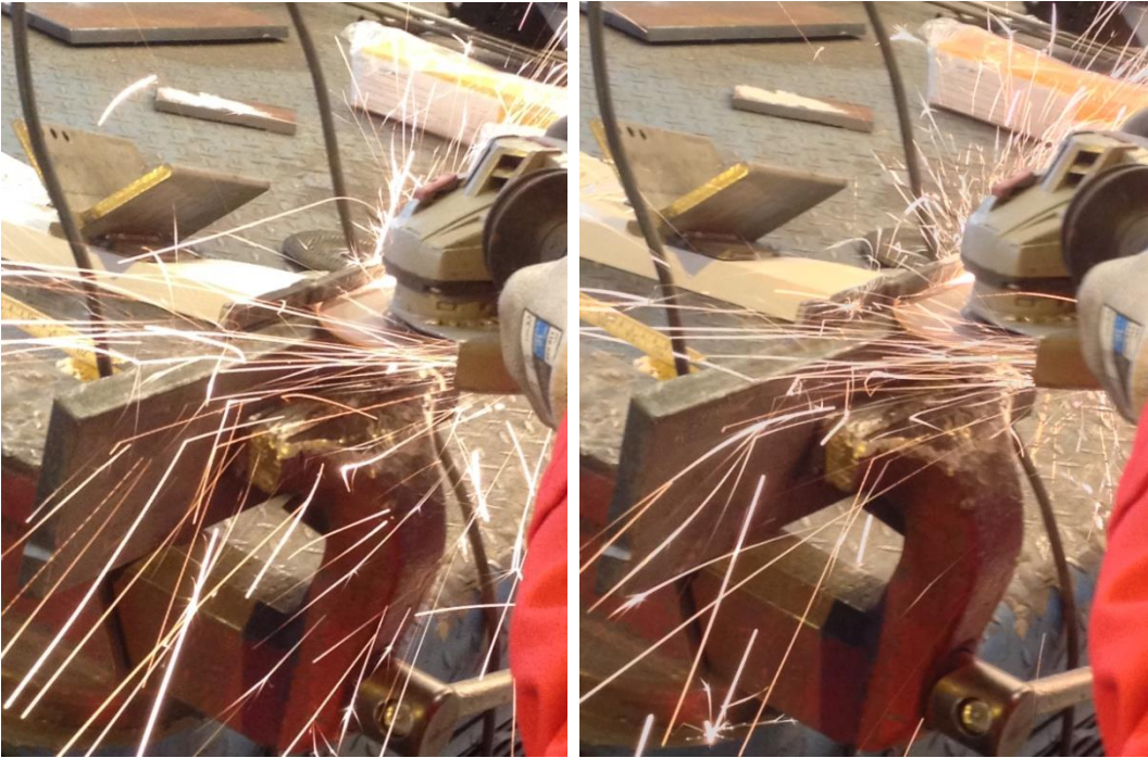
Figure 5-10 & Figure 5-11 Cutting of specimens
