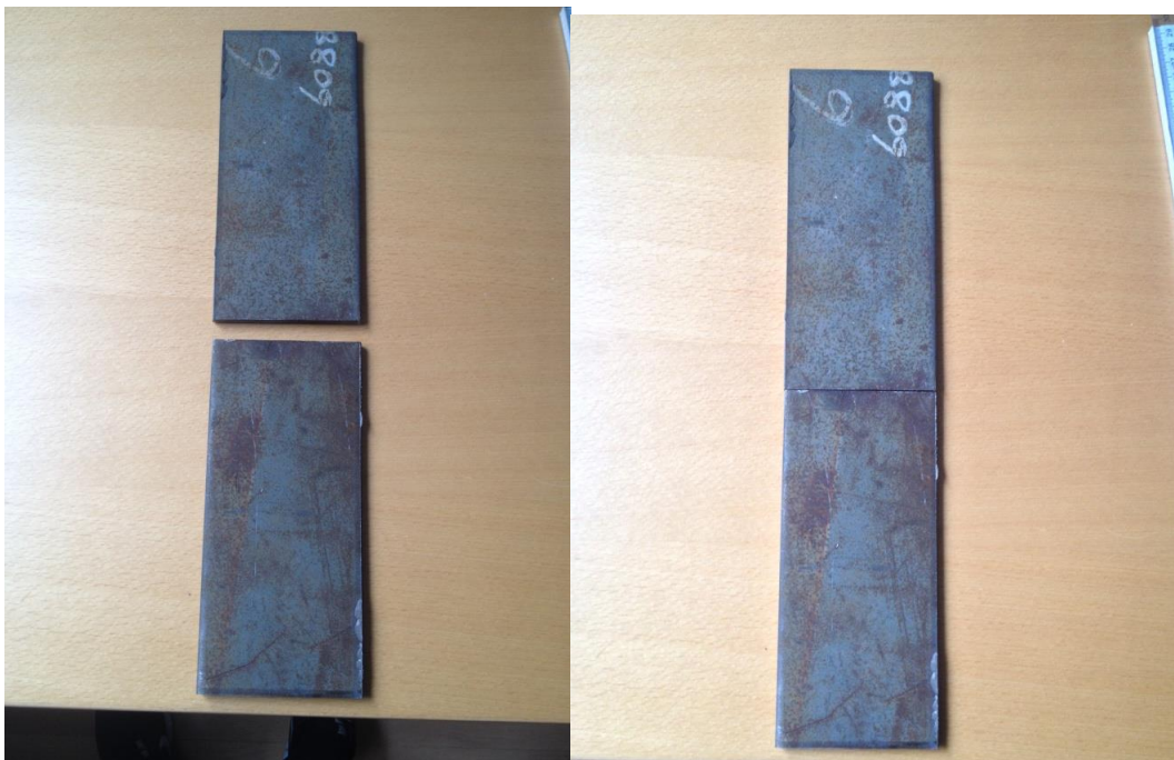
Figure 5-1 & Figure 5-2 Pre weld steel plates
