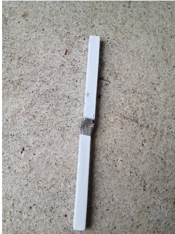
Figure 7-11 Displaced specimen after weld
