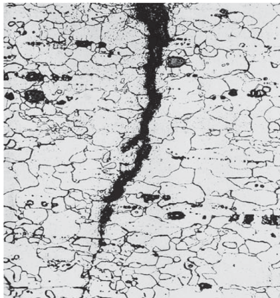
Figure 2.4: Corrosion-fatigue fracture through mild steel sheet, resulting by fluting of the sheet in flue gas condensate [3]
