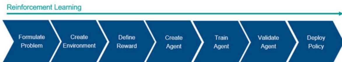
Figure 3.4: Reinforcement Learning workflow using MATLAB RL Toolbox [12]
