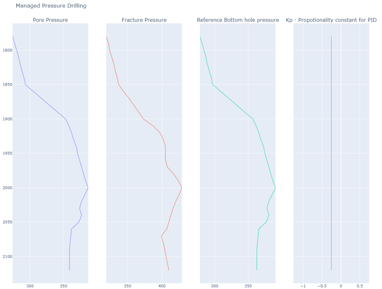
Figure 6.13: Pore Pressure, Fracture Pressure, Reference BHP, Kp from left to right - Case without oscillations reward
