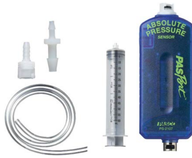
FIGURE 3.8: Absolute pressure sensor and its connections
