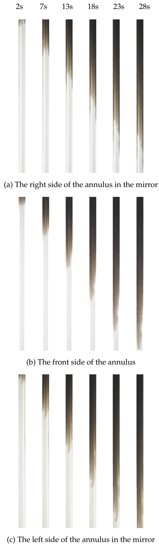
FIGURE 4.9: Fluid displacement for At = 0 and v = 25 mm/s
