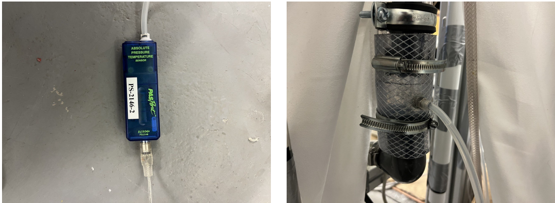
FIGURE C.10: Pressure sensor and connecting tubes
