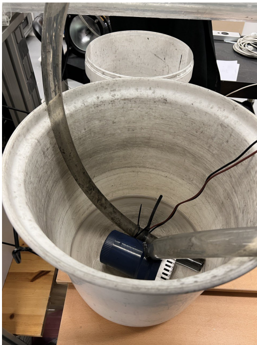
FIGURE C.7: Heavy fluid reservoir, pump and power supply
