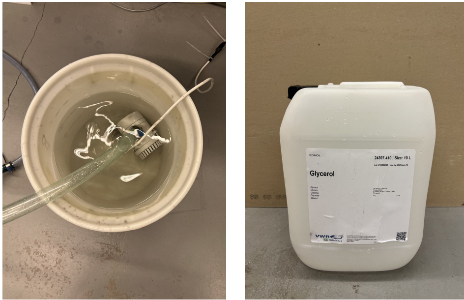
FIGURE D.2: Container and pump for viscous solution, and glycerol
