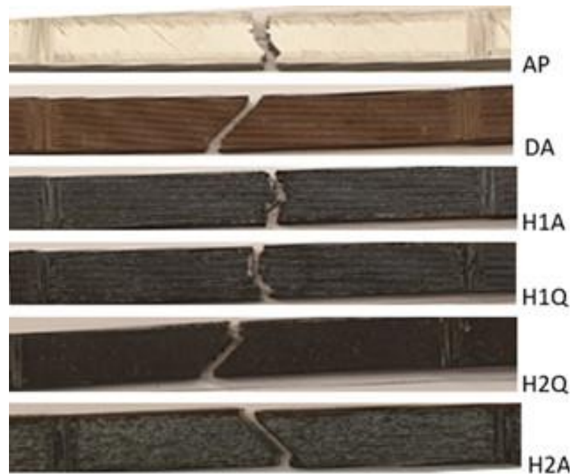
Figure 14. Fracture profile of material failure during the tensile test.
